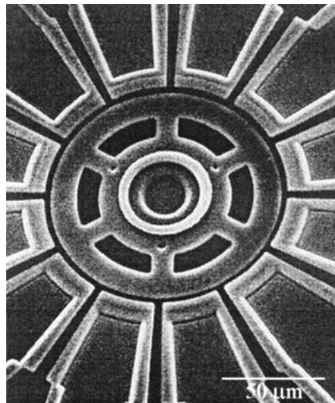
FIGURE 16.2 SEM micrograph of a harmonic side-drive (wobble) micromotor. (From Mehregany, M. et al., 1990, in Proc. IEEE Micro Electromechanical Systems , pp. 1–8, IEEE, New York. With permission.)
