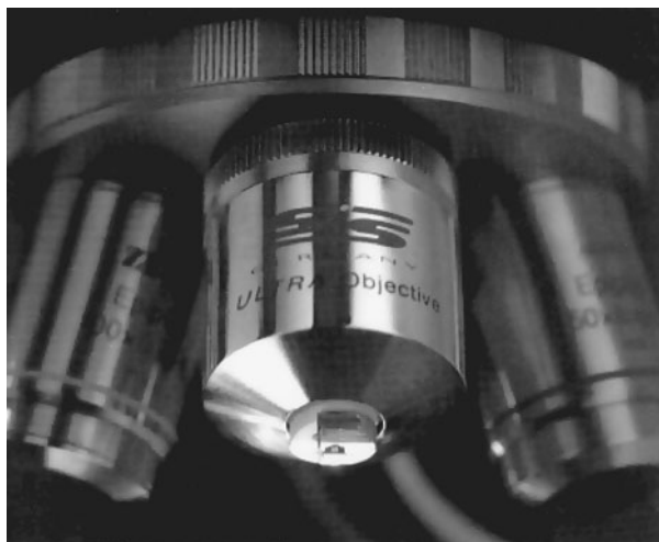
FIGURE 2.30 The stand-alone microscope Ultra-Objective™ from SIS. (Courtesy of SIS. With permission.)
