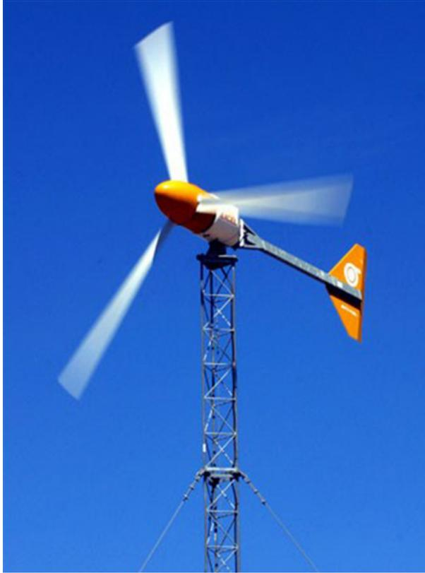
**Figure 2.2.** Image of a small-scale HAWT.
