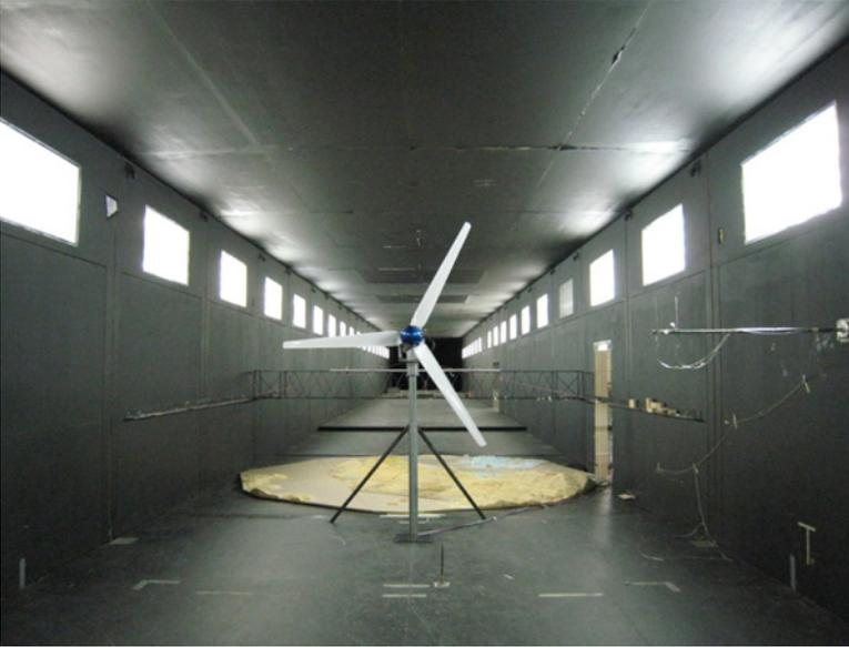
**Figure 5.18.** Wind tunnel test setup of a small HAWT [17].
