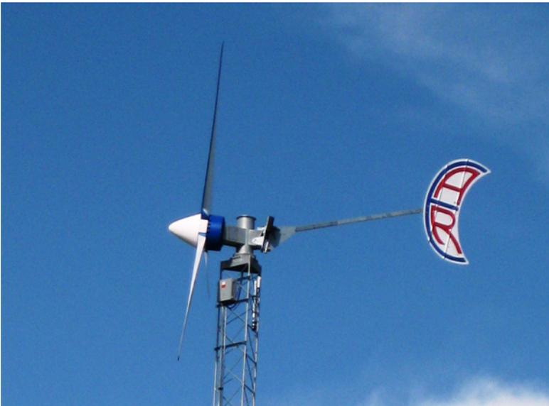
**Figure 1.5.** Close-up photograph of a propeller HAWT.
