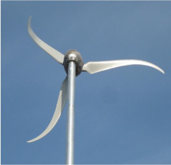
**Figure 1.6.** Rotating HAWT rotor with contoured blades.
