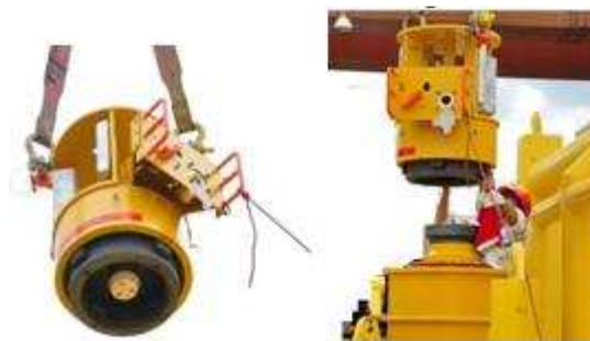
Fig.4. Pressure cap installation test
