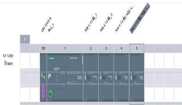
Fig.2. The connection between CPU and extension modules
