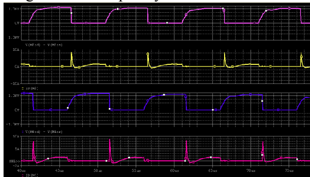
Figure5. The main switch tube S_1 and S_2 of drain-source voltage waveform and the drain current simulation waveform
