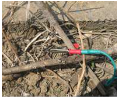
Figure 4 The retracting lead wire caught in the stick
