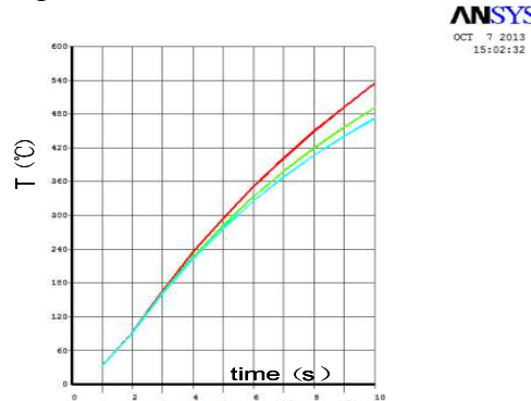
Fig. 7 The temperature curves of three nodes at different location of grounding resistor.
