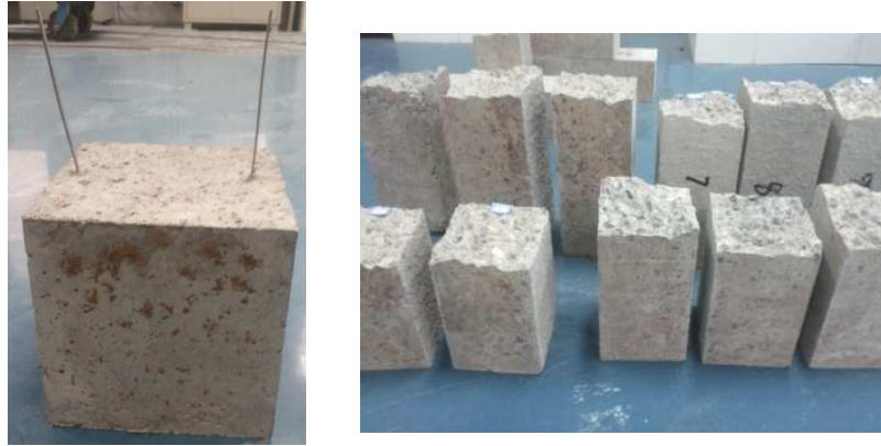
Fig.2 CFCC samples for electrical resistivity and rupture strength tests
