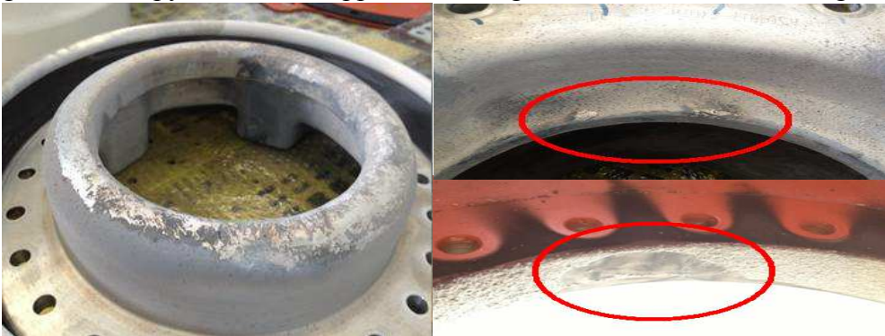
Fig.3 The empyrosis of the ambilateral fixed metal parts of the support insulating tube
