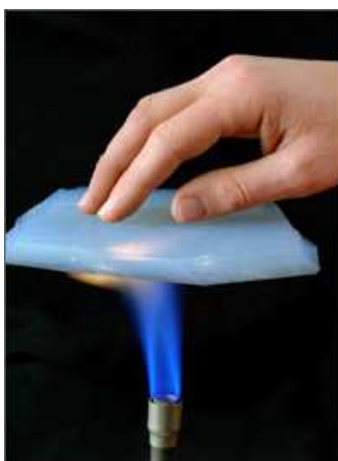
Fig. 1. Excellent thermal insulation property of nano pore structure [2]
