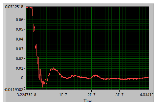
Fig. 9 800kV capacitive voltage divider step response waveform figure(wavefront with oscillation)
