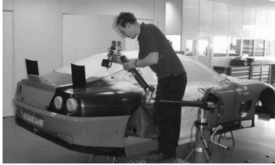
Figure 7.5. Advanced CFD Model X with a Faro arm is used to capture half of the Ferrari 550 Maranello body. Copyright © Advantage CFD, Brackley, Northamptonshire, UK, www.advantage-cfd.co.uk . Reproduced with permission.
