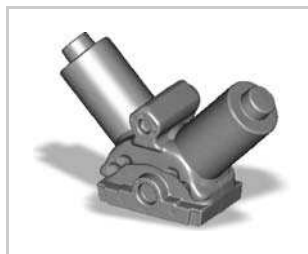
Figure 7.3. Reverse-engineered model of urethane molds of the internal cavities from the SB2 engine. Copyright © Richard Childress Racing Enterprises, Inc., Welcome, NC, USA, www.rcrracing.com . Reproduced with permission.
