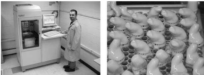
Figure 9.9. An SLA system and the hearing instrument shells it produces. Copyright © GN ReSound Corp., Bloomington, MN, USA, http://205.242.218.80%20/home.aspx . Reproduced with permission.
