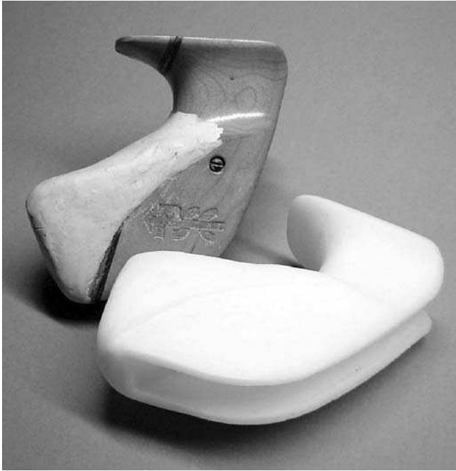
Figure 5.8. Scanned archery handle and an FDM reproduction
