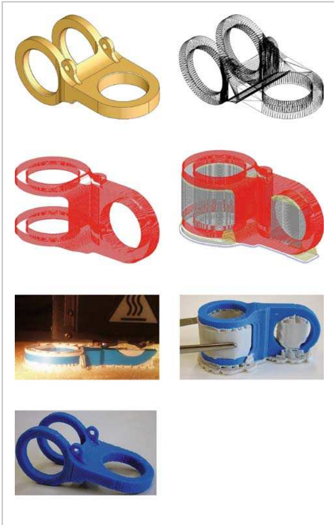
Figure 5.2. The basic RP process (FDM)
