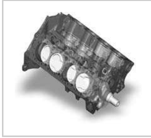
Figure 7.4. The completed digital model of the SB2 engine block with rotating assembly. Copyright © Richard Childress Racing Enterprises, Inc., Welcome, NC, USA, www.rcrracing.com . Reproduced with permission. A color reproduction of this figure can be seen in the Color Section (pages 219–230).
