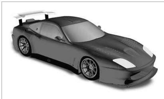
Figure 7.7. Ferrari 550 Maranello body reverse engineered in Geomagic Studio software and assembled and visualized in Pro/E software
