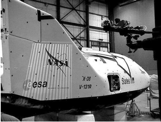
Figure 8.13. Scanning the outer side
