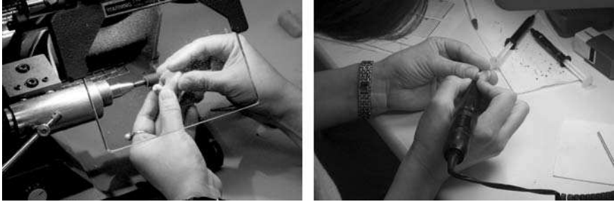
Figure 9.7. Traditional process using manual sculpting and drilling. Copyright © GN ReSound Corp., Bloomington, MN, USA, http://205.242.218.80%20/home.aspx . Reproduced with permission.
