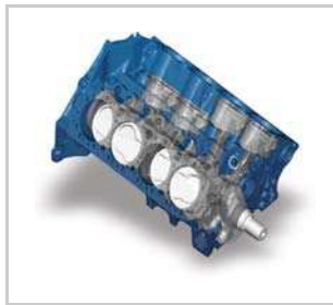
Figure 7.4. The completed digital model of the SB2 engine block with rotating assembly. Copyright © Richard Childress Racing Enterprises, Inc., Welcome, NC, USA, www.rcrracing.com . Reproduced with permission.
