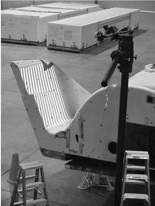
Figure 8.12. Scanning the inner side of the wing
