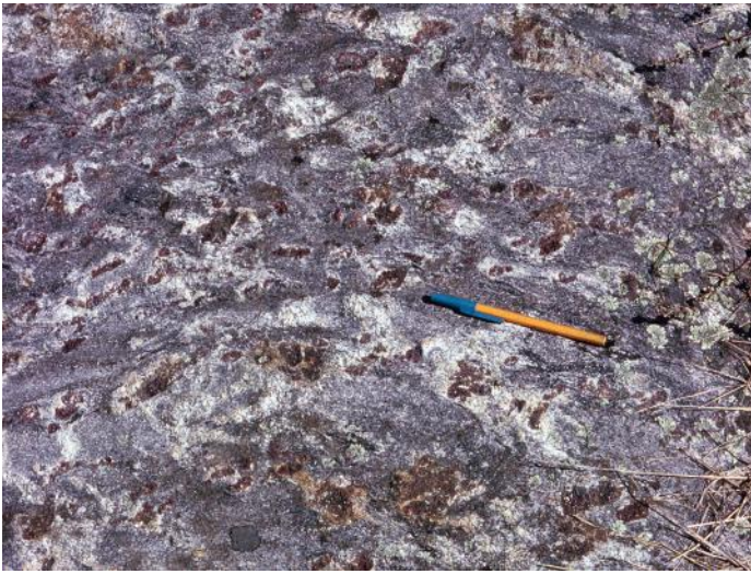
Figure 2.13 Gneissic biotite schist at sillimanite – K-feldspar – garnet – cordierite grade. All of the muscovite and some of the biotite has broken down to make anhydrous phases. Lacking most of its original micas, the rock is more gneissic than typical schists at lower grade. In addition, partial melting has produced coarse leucosomes (the light colored areas, Chapter 21) of segregated, crystallized melt in which grew large garnets. The leucosomes seem to be randomly arranged, suggesting that this rock was not deformed very much after the melt crystallized. Ware, Massachusetts, USA.
