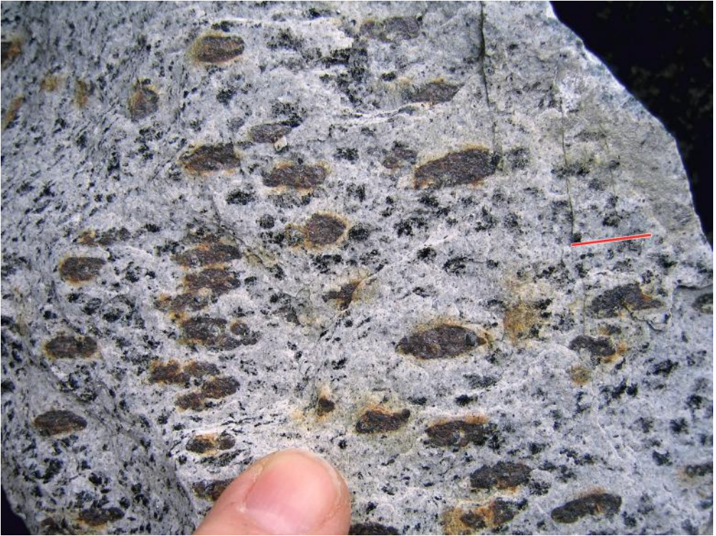
Figure 15.13 A somewhat weathered, fine-grained felsic gneiss, that has flattened and elongate, rusty-weathering pyrite grains. The pyrite grains define both the rock lineation, parallel to the red line, and, with minor biotite, the foliation. The foliation surface occupies the entire center of the image. Rissa, outer Trondheimsfjord, Sør Trøndelag, Norway.
