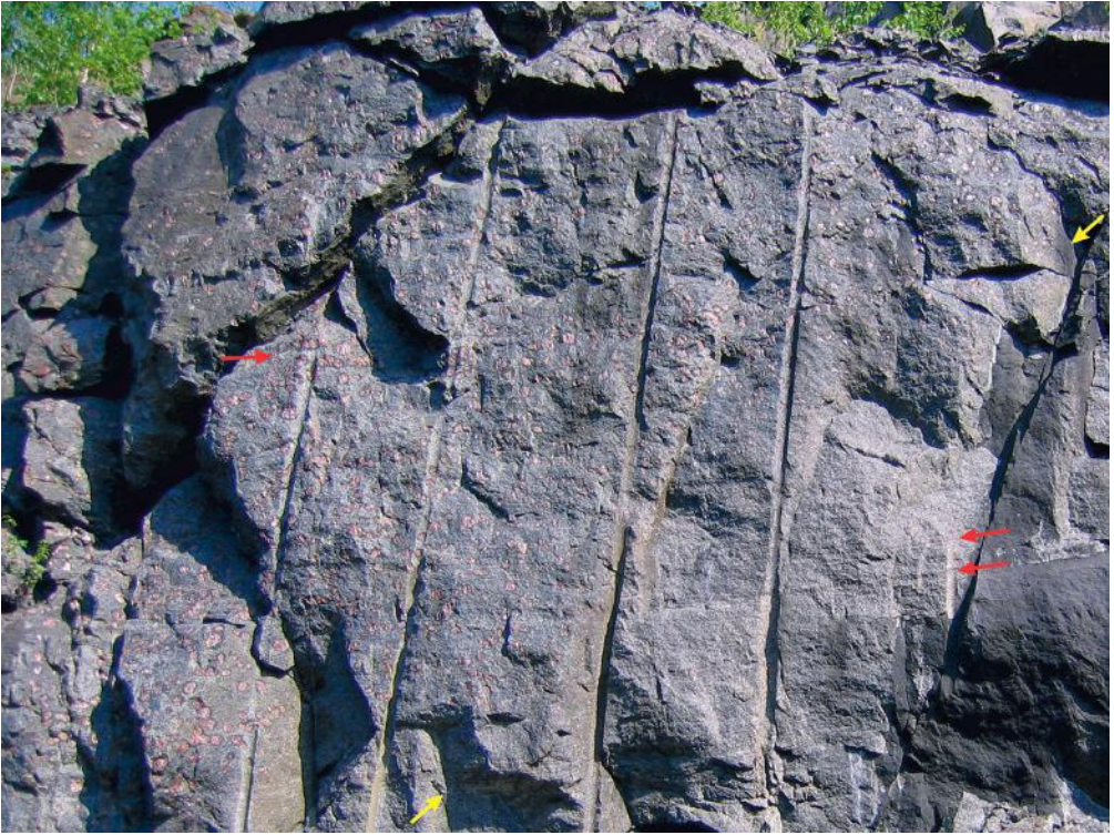
Figure 20.13 Quarry face at an abandoned garnet mine. The garnet amphibolite ore rock is to the left of the boundary indicated by the yellow arrows. The precursor rock, to the right, is layered olivine gabbro that was metamorphosed to granulite facies conditions. The transition zone between the two is about 2 m wide, over which metamorphic garnets less than 0.2 mm in diameter in the gabbro gradually decrease in number, and increase in size, to greater than 10 cm in diameter. Cumulate layering, indicated by red arrows, extends from the gabbro into the garnet amphibolite, indicating that the precursor rock transformed directly to garnet amphibolite with little deformation. The garnet amphibolite formed during infiltration metasomatism by an aqueous fluid at upper amphibolite facies conditions. The major element compositions of the gabbro and garnet amphibolite are nearly identical, except of course for H_2O . However, some trace elements in the garnet amphibolite are dramatically enriched or depleted, and inhomogeneous, compared to the gabbro (Hollocher, 2008; Morgan and Hollocher, 2011), indicating channelized fluid flow. North River, New York, USA.
