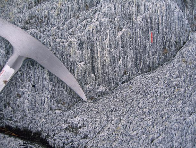
Figure 15.11 Tonalitic gneiss having a vertical cleavage (the flat wall parallel to the plane of the hammer head and handle) and strong vertical mineral lineation on the cleavage surface (red line). The rock contains mostly plagioclase and quartz, with only 10% biotite and other minerals. The strong lineation is made up of long ribbons of quartz about 1 mm wide and strings of recrystallized plagioclase and biotite. The rock surface below and to the right of the hammer point is approximately perpendicular to the foliation and lineation, so the lineation is seen almost end-on (just looks like black-and-white speckles) and the foliation is clearly weak. Almvikneset, Trondheimsfjord, Sør Trøndelag, Norway.
