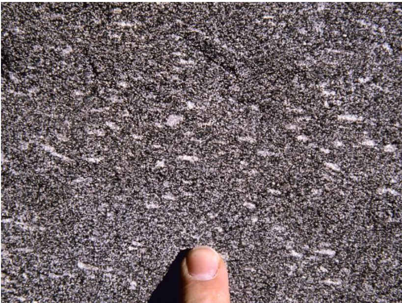
Figure 9.12 Fine-grained amphibolite metamorphosed to amphibolite facies conditions, with elongate, white, monomineralic spots of plagioclase. These are interpreted to be recrystallized plagioclase phenocrysts, based on their pure plagioclase mineralogy, and the nearby presence of apparently relict igneous plagioclase cores in some particularly large plagioclase porphyroclasts (Fig. 25.1C, D). Quabbin Reservoir, Massachusetts, USA.
