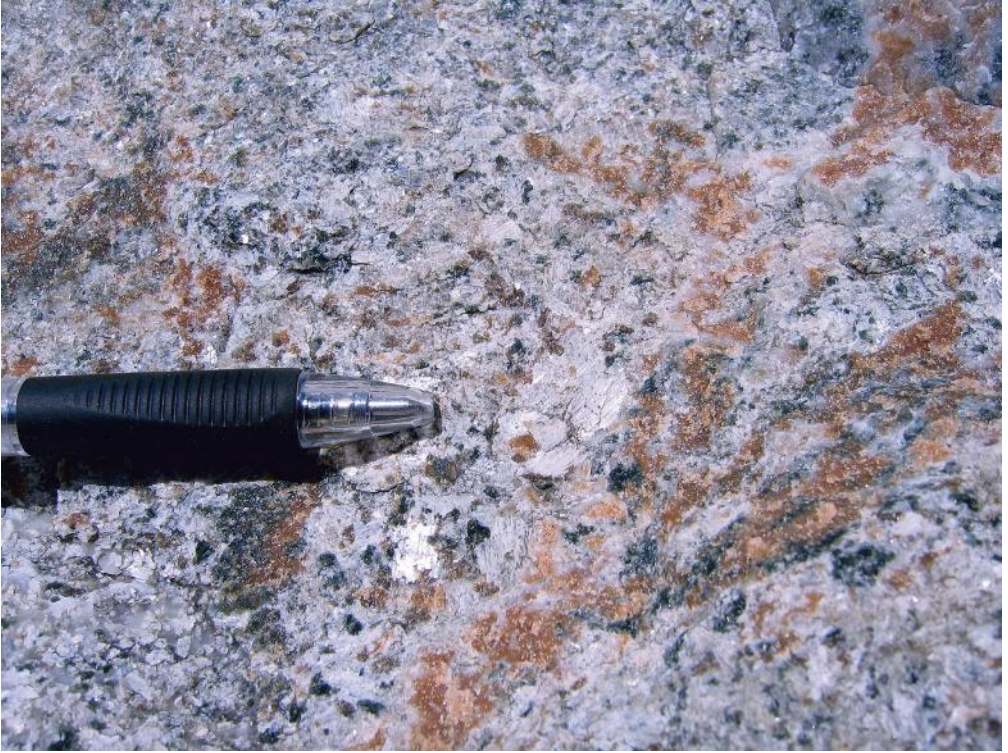
Figure 5.11 Calc-silicate rock that occurs at the contact between diopside – quartz marble and metamorphosed gabbro, which are about a half meter away to the left and right, respectively. The marble and gabbro themselves have metamorphic mineral assemblages characteristic of the upper amphibolite facies. The calc-silicate rock shown here is composed of orange grossular-andradite garnet, dark-green diopside, and white scapolite and wollastonite. Where fresh, scapolite and wollastonite can be difficult to tell apart in the field. However, the greater solubility of wollastonite causes the initially rough surfaces to become smooth. The white material in most of the image is scapolite, but the smooth-looking white and gray material in the lower left corner is wollastonite. Strangely, the wollastonite-bearing assemblage shown here is characteristic of high-temperature, low-pressure contact metamorphism, not regional amphibolite facies conditions (Figs. 1.1, 5.1). At this outcrop common marble is abundant, and this anhydrous calc-silicate assemblage occurs only at the gabbro-marble contact. It is possible that the calc-silicate rock was originally formed when the gabbro intruded at low pressure, forming the dry calc-silicate contact metamorphic assemblage. This assemblage then survived subsequent upper amphibolite facies regional metamorphism. Comstock, Adirondacks, New York, USA.
