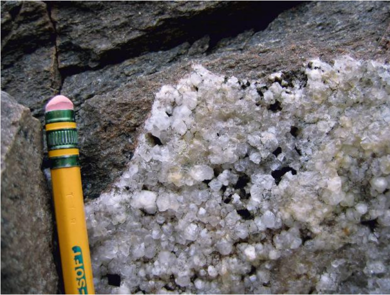
Figure 19.6 Terminated quartz crystals partially filling a vein in tonalitic gneiss. The fact that the quartz occurs as terminated crystals indicates that the fracture was never completely filled with quartz, and was never forced closed by lithostatic pressure. This means that the vein was deposited at a relatively shallow depth where the rocks were strong enough to hold the walls apart until the vein reached the surface. These crystals, especially near their terminations, are quite transparent, but typically vein quartz is loaded with fluid inclusions which make it look white. Lensvik, Trondheimsfjord, Sør Trøndelag, Norway.
