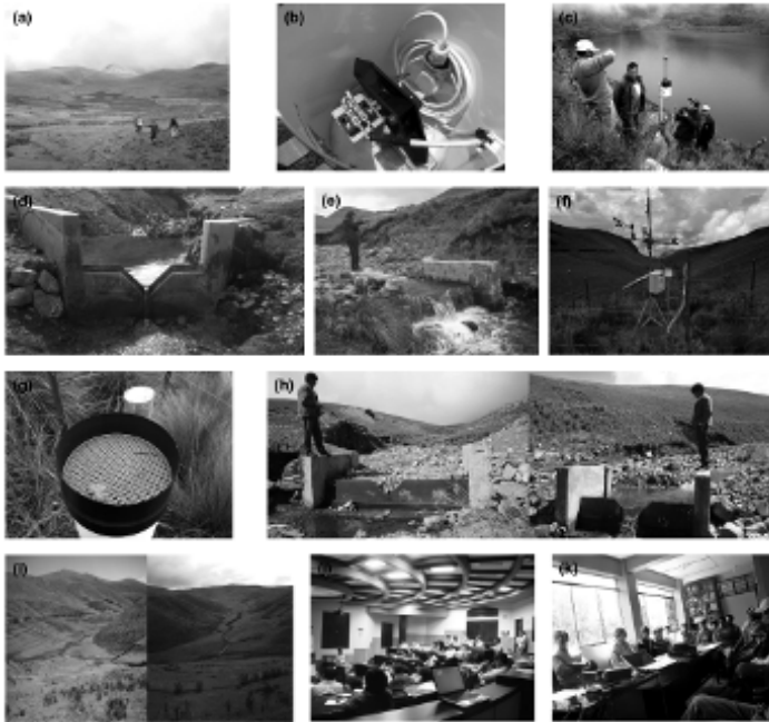
Fig. 6.25. Pictures depicting several steps in the iMHEA protocol: (a) Selection of monitoring catchments in Tambobamba, Peru, by a group of hydrologists, local partners and users of land and water. Photo: Boris Ochoa-Tocachi, 2011. (b) Example of a tipping bucket rain gauge with a resolution of 0.2 mm installed in Lloa, Ecuador. Photo: BOT, 2014. (c) Local partners of iMHEA installing a rain gauge in Piura, Peru. The rain gauge accuracy is revised using static and dynamic calibration methods on a regular basis. Photo: BOT, 2012. (d) A weir located at the outlet of an iMHEA catchment in Ica, Peru. The V-shaped section of the weir allows an accurate monitoring of low flows. Photo: Junior Gil-Rios, 2015. (e) A weir located at the outlet of an iMHEA catchment in Huaraz, Peru. The composite triangular-rectangular section allows the monitoring of high flows. Photo: JGR, 2014. (f) A weather station is located at a central location between the iMHEA catchments in Lloa, Ecuador. The monitoring of several climatic variables, in this case temperature, relative humidity, solar radiation, wind velocity and direction and rainfall, allows for a more accurate calculation of evapotranspiration. Photo: BOT, 2014. (g) Example of a tipping bucket rain gauge in Lloa, Ecuador, with some litter retained in the filter. Photo: BOT, 2014. (h) Hydrological monitoring of two catchments under different levels of conservation/alteration in Cochabamba, Bolivia. A local farmer contrasts visually (left) a highly degraded catchment produced by cultivation and overgrazing, against (right) a relatively conserved catchment situated closely to the former. In what we refer to as the 'Placebo iMHEA effect', local users recognize the relevance of monitoring impacts, even before seeing any data. Photos: Luis Acosta, 2012. (i) Highly seasonal catchment in Tambobamba, Peru. In puna, the landscape is markedly different during the (left) dry season and the (right) rain season. Photos: BOT, 2012, 2013. (j) An International Course on Andean Hydrology and Hydrological Monitoring organized by Nature and Culture International, CONDESAN, the University of Piura, Peru, and iMHEA in Piura in 2013. Photo: BOT, 2013. (k) A group of farmers in a meeting with local decision makers and hydrologists from iMHEA in Pacaipampa, Peru. Photo: BOT, 2012.
