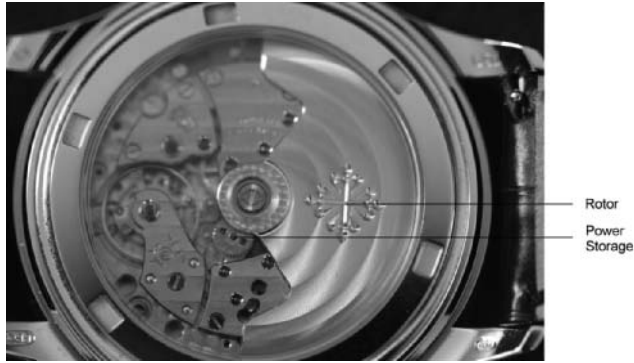
Figure 9.6 Automatic winding movement mechanism
