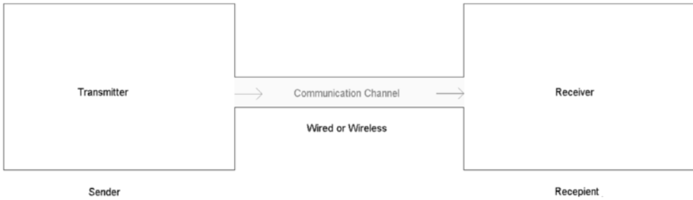
Figure 2.1 Block diagram of a basic communication system
