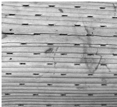
Figure 2.19 Incising cuts in pressure treated wood
