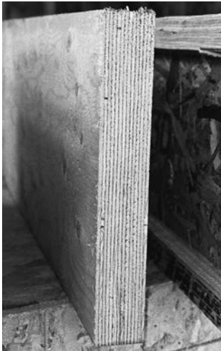
Figure 2.10 Laminated veneer lumber (LVL) cross section
