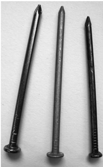
Figure 9.5 Common bright, box galvanized, sinker coated, common nails (from left to right)
