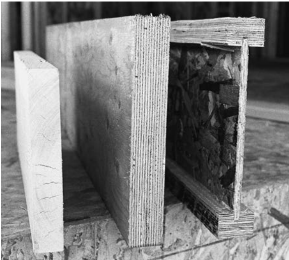
Figure 4.3 Sawn, composite, and I-joist
