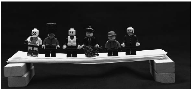
Figure 5.3 Paper beam with layers (a) unglued and (b, c) glued (Lego™ figures courtesy Peter McMullin)
