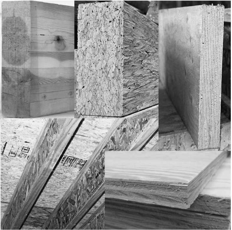
Figure 2.8 Engineered wood products. From top left, clockwise: glued laminated timber, PSL, LVL, I-joint, and structural panel
