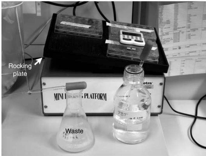
Fig. 3. Rocking platform and other equipment required for antibody staining of imaginal discs. See text for further information.
