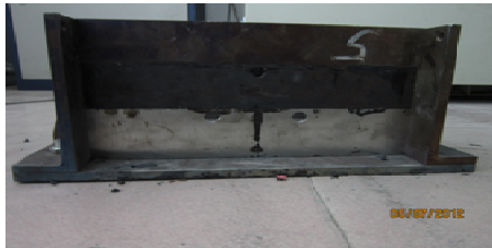
Fig.4 Two layer combined structure boards
