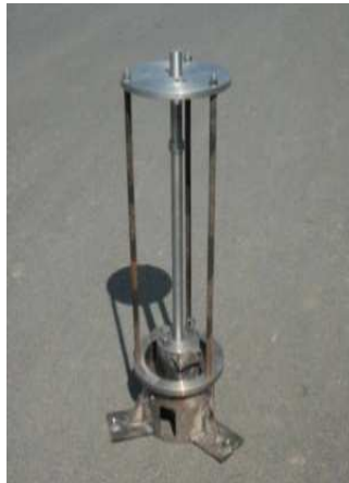
Figure 8. Penetrating Strength Detector of Shallow Pavement
