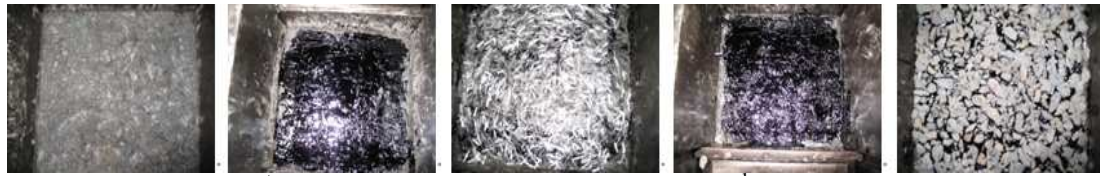
a. Prepare base b. 1 st layer of asphalt c. fiber d. 2 nd layer of aspha e. spread gravel Fig. 1. Process of Laboratory Production
