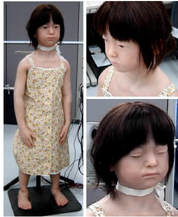
Fig. 5. The developed android robot named “Repliee R1.” Left: External appearance. Upper Right: Head appearance. Lower right: Head appearance with eyes closed.
