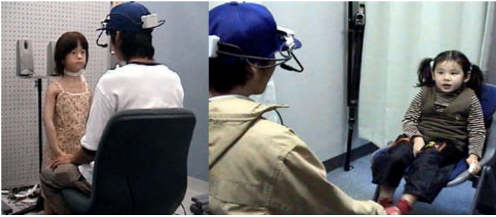
Fig. 8. Experimental room. A subject mounting an eye mark recorder has a brief conversation with the android (Left) and the girl (Right.)
