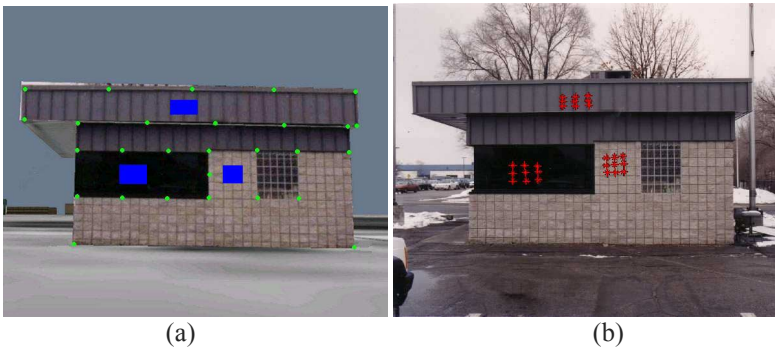
Fig. 5. An example of mapping virtual objects to an image of real scene. (a) shows the virtual image containing the control points and three virtual objects. (b) shows a real view image with mapped virtual objects shown in “RED.”
