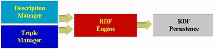
Fig. 4. Architecture of the RDFCore system
