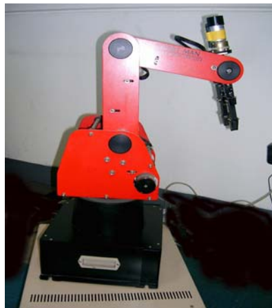
Fig. 6. Modeled two degree-of-freedom robot manipulator
