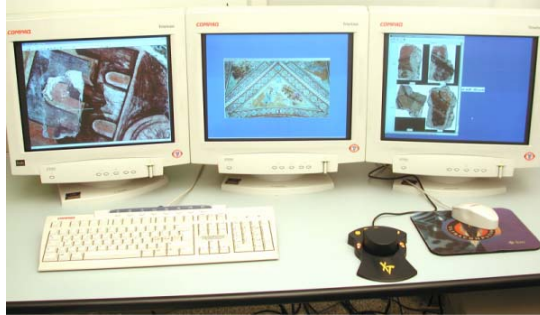
Fig. 1. The workstation for virtual aided recomposition. The left-side monitor represents the working area where fragments images are placed. On the other ones a scaled version of the whole fresco and a virtual container are shown
