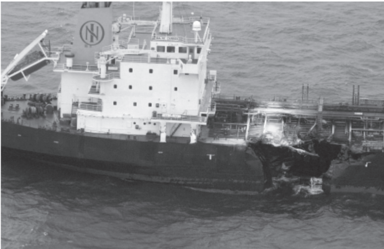
Figure 8.2 The oil released from tank no. 6 of the m/v Baltic Carrier (DMA 2001).
