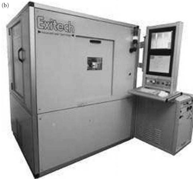
Figure 3.20 Excimer laser: (a) schematic; (b) Exitech M5000 micromachining tool. (Source: Adrian Baughan, Exitech Ltd, Oxford, UK)
