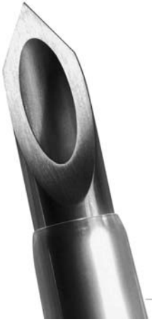
Figure 17.4 Intravenous catheter drilled using a pulsed Nd:YAG laser. (Source: Mo Naeem, GSI Lumonics, Rugby, UK)
