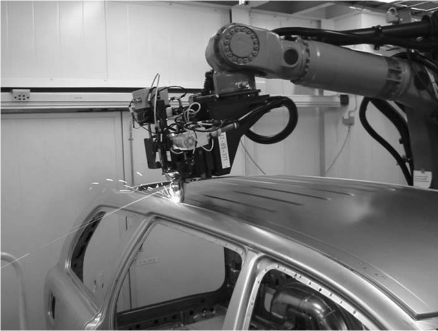
Figure 2.4 Roof edge laser welding of the Volvo XC90. (Source: Johnny Larsson, Volvo Car Corporation, Gothenburg, Sweden)
