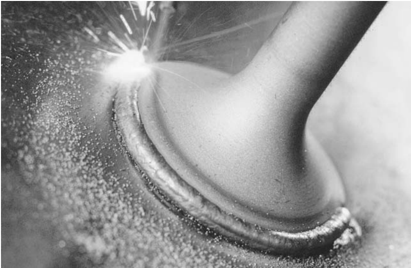
Figure 12.1 CO 2 laser beam cladding of a valve rim with cobalt-based hardfacing powder. (Source: Tero Kallio, Lappeenranta University of Technology, Finland)
