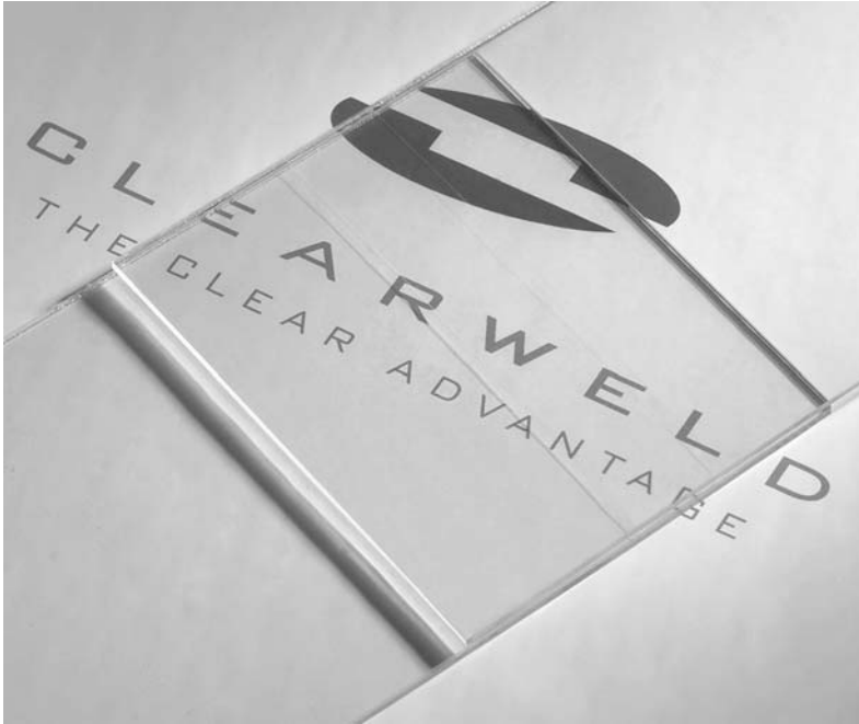
Figure 13.6 A lap joint made in PMMA using the Clearweld™ process. (Source: L.P. Freider III, Gentex Corporation, Carbondale, PA, USA. Clearweld is a registered trademark of TWI)
