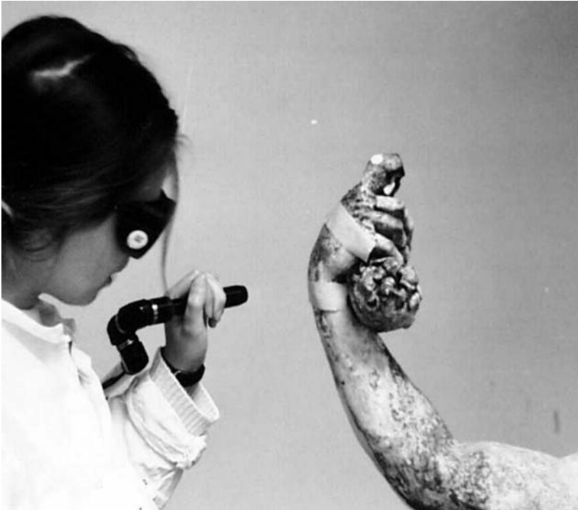
Figure 1.10 Restoration of a statue by pulsed Nd:YAG laser cleaning. (Source: Paolo Salvadeo, Quanta System SPA, Milan, Italy)
