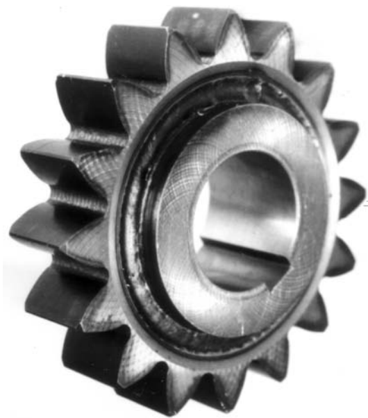
Figure 18.2 Gear–hub assembly made using laser welding and laser hardening
