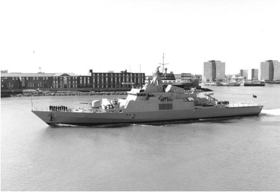
Figure 2.6 Corvette constructed from laser-cut plates. (Source: Ian Perryman, Vosper Thornycroft, Southampton, UK)
