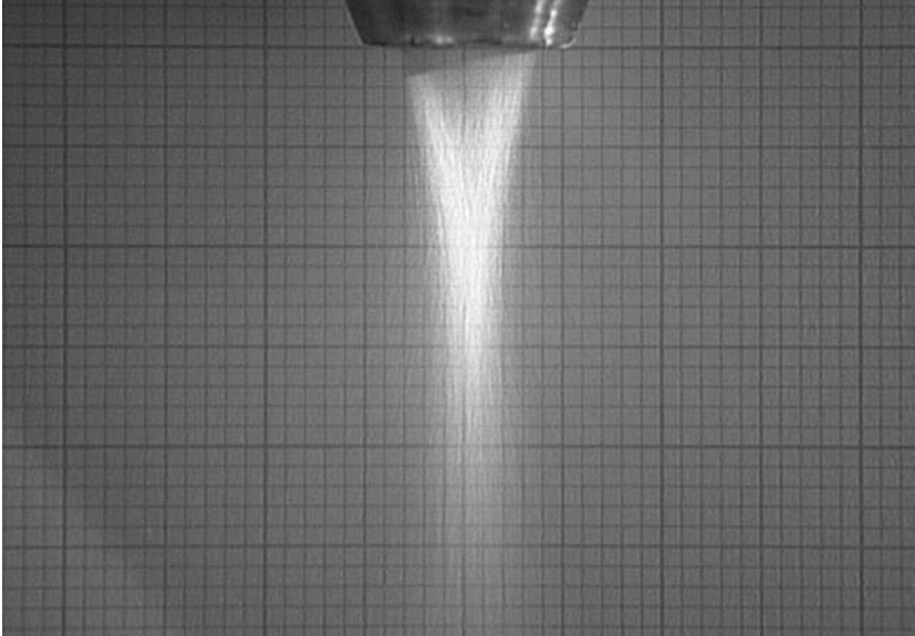
Figure 12.3 Coaxial alloy powder feed. (Source: Antti Salminen, Lappeenranta University of Technology, Finland)
