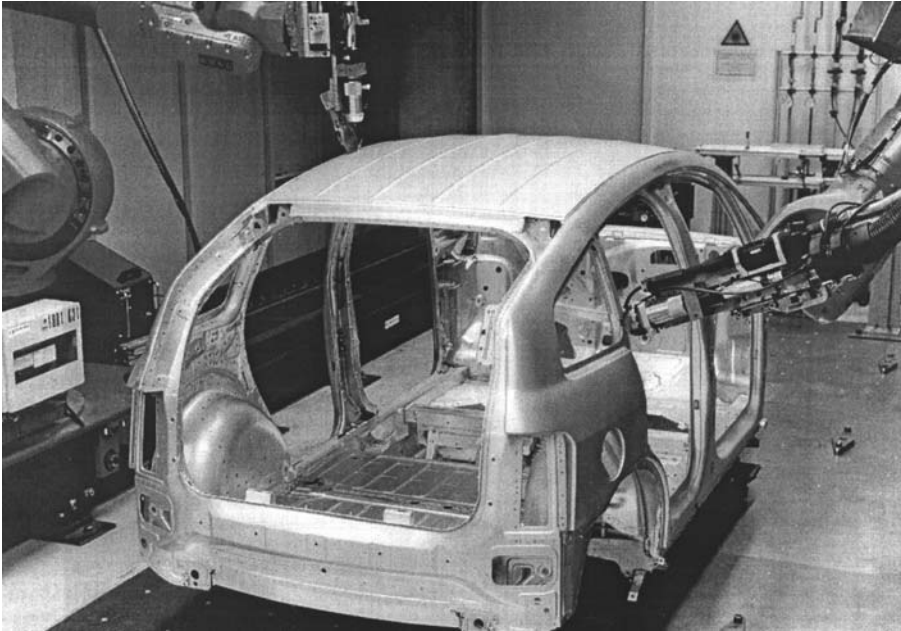
Figure 1.5 Audi A2 aluminium alloy spaceframe. (Source: Jens Christlein, Audi AG, Neckarsulm, Germany)
