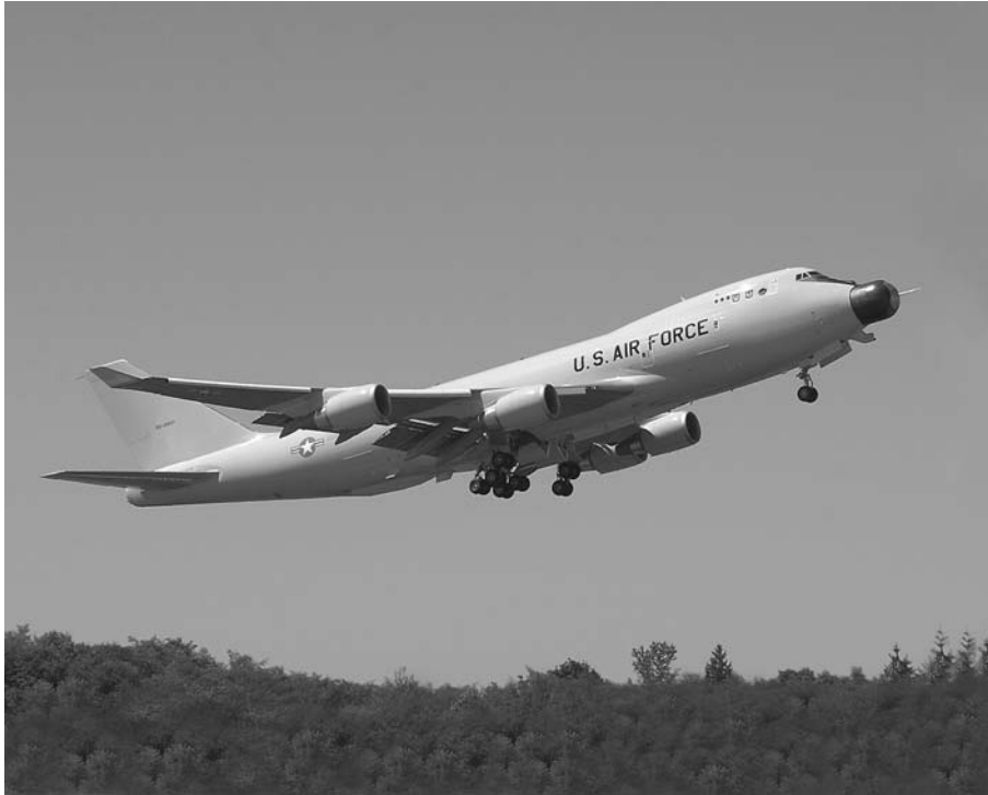
Figure 2.5 Airborne laser: high energy chemical oxygen iodine laser (COIL) carried aboard a modified Boeing 747-400F freighter. (Source: Mary Kane, Boeing, Seattle, WA, USA)
