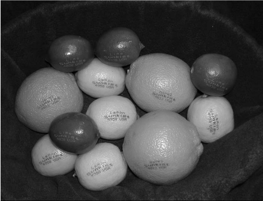
Figure 15.6 Fruit marked using a sealed CO 2 laser and a dot matrix format created by a high speed scanner. (Source: David Belforte, Industrial Laser Solutions, Sturbridge, MA, USA)
