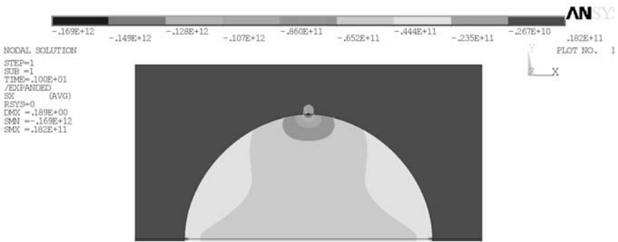
Figure 2.80. Horizontal stresses in the homogenisation problem \chi^{12}
