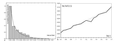
**Figure 9.8.** Fitting the Weibull model to the time until breaking of aluminium specimens submitted to high amplitude sinusoidal loads in fatigue tests: a) Lifetable estimate of the survivor function with Weibull estimate (solid line); b) Log-cumulative hazard plot (solid line) with fitted regression line (dotted line).
