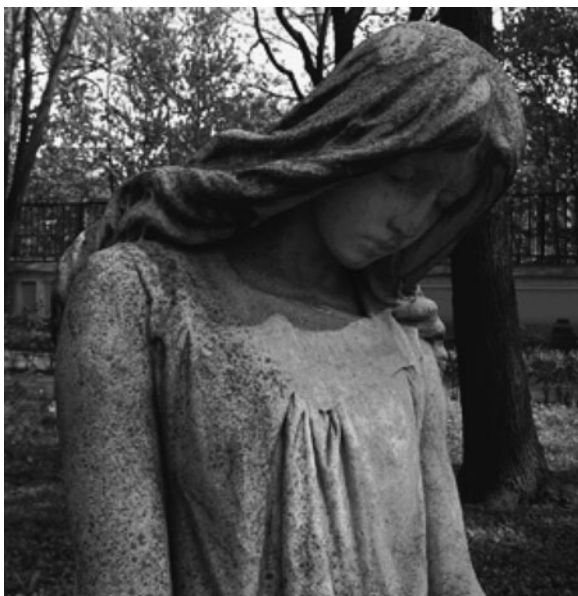
Fig. 2 Micromycetes colonies on Carrara marble sculpture (Saint Petersburg) in a year after treatment by organotin and quaternary ammonium biocides
