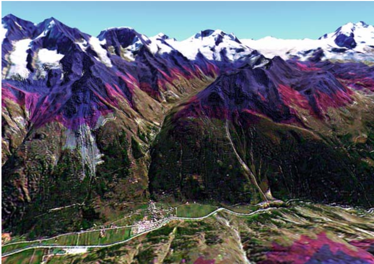
Fig. 14.1 The village of Täsch and the Mischabel Group in the Matter Valley, Valais Alps, Switzerland, with numerically simulated permafrost distribution ( blue ; red = uncertainty zone and probably warm/degrading/already thawed permafrost). Note dams for rock fall protection on left and debris flow on right slope above village. In 2001, a debris flow from a moraine lake in marginal permafrost of the lateral valley ( centre of image ) caused heavy damage to the village (satellite imagery: © ESA/Eurimage, CNES/Spotimage, swisstopo/NPOC; permafrost simulation/visualization: S. Gruber, S. Biegger, University of Zurich)
