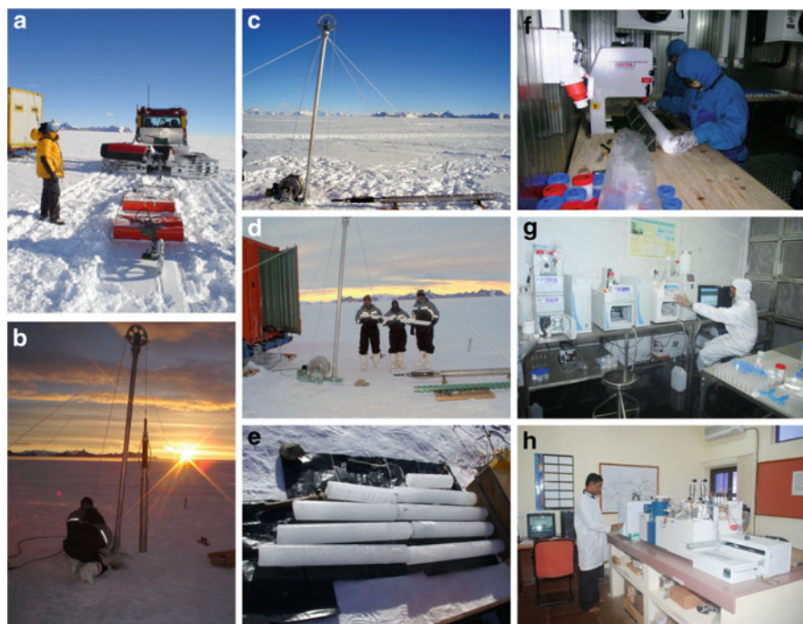
Fig. 5.2 Field photographs of the Indian ice core project and the laboratory activities at NCAOR. (a) Ground Penetrating Radar survey for site location; (b) ice core drilling in progress; (c) the drill set up; (d) team with the first ice core; (e) ice cores ready for transport; (f) samples processing at -15^{\circ}\text{C} cold room facility; (g) clean room facility and ion chromatography system; (h) isotope ratio mass spectrometer facility
