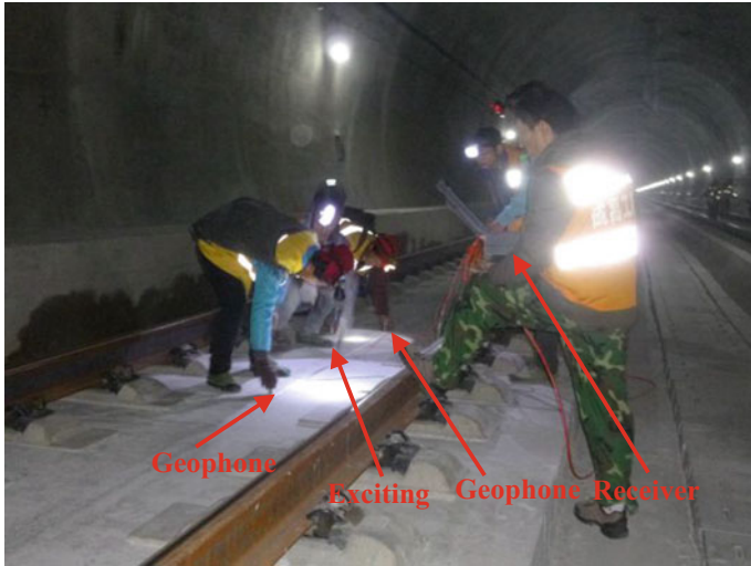
Fig. 2 The way to work of Landsonar
