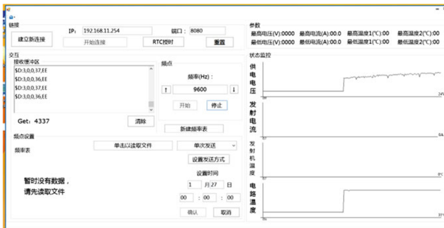
Fig. 6 Diagram of control software in the transmitter host computer
