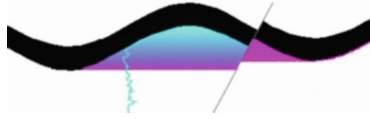
Fig. 6.48 Simple analytical petroleum trap filled to the spill point and leaking through a fault with a lower P_{CT} than the caprock (from Ringrose et al. 2000)
