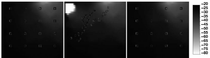
Fig. 2 Piezometric head fields at the end of the three stress periods and spatial location for T data, c data at three snapshots and h data at three periods ( from left to right )
