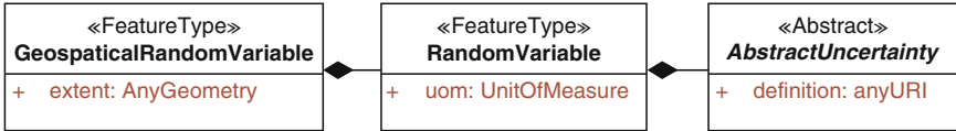
Fig. 12 Three layered implementation of UncertML. At it’s simplest, UncertML only encodes the values of an uncertainty type. A ‘RandomVariable’ type adds a link to a phenomena and its units of measure and a ‘GeospatialRandomVariable’ adds further detail with an attached geometry. These random variable types are not included in UncertML and represent only one possible implementation
