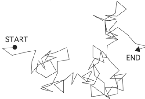
Fig. 2.3. Example of a Monte Carlo simulation for 100 steps of Brownian motion of a particle. Each time step, the particle jumped a unit distance in a random direction
