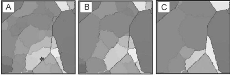
Fig. 3.3.3 Example run showing isotropic surface energy driven subgrain growth. Greyscale scheme shows relative misorientation from one crystallographic orientation (marked as black star) in greyscale; black lines signify grain boundaries with >15^\circ misorientation; (a-c) results at model time steps 1500, 2500, 6000 (modified after Piazzolo et al., 2004). 🌀 EXPERIMENT 6
