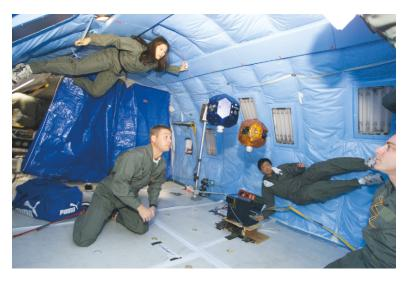
FIGURE 5.2. THE SPHERES PROJECT AT MIT: TESTING AUTONOMOUS ROBOTS IN "0-GRAVITY"
