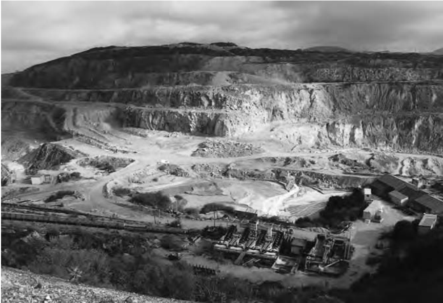
Fig. 3.2 View across Melbur pit. China clay washed from the working face, using high pressure monitor hoses, enters a pumping and sand separation plant.
