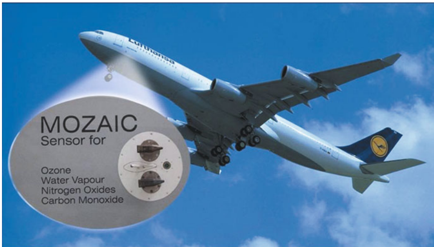
Fig. 2.4 Airbus A340 equipped with MOZAIC-humidity device. Inlet system is mounted at the outside skin of the aircraft close to the cone
