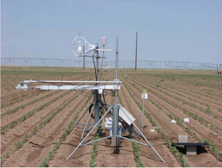
FIGURE 5.3 EC SEBS over an emerging cotton field. EC is oriented to due south; the lateral irrigation system is in the background.
