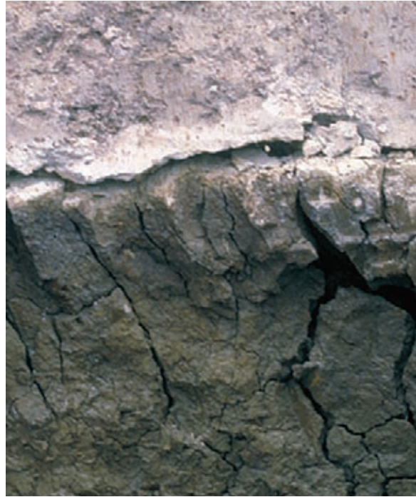
Figure 6.13. A sodic soil in Tasmania, Australia, that lacks aggregation and has problems with waterlogging when wet and with hardsetting when dry. Photo by Richard Doyle.
