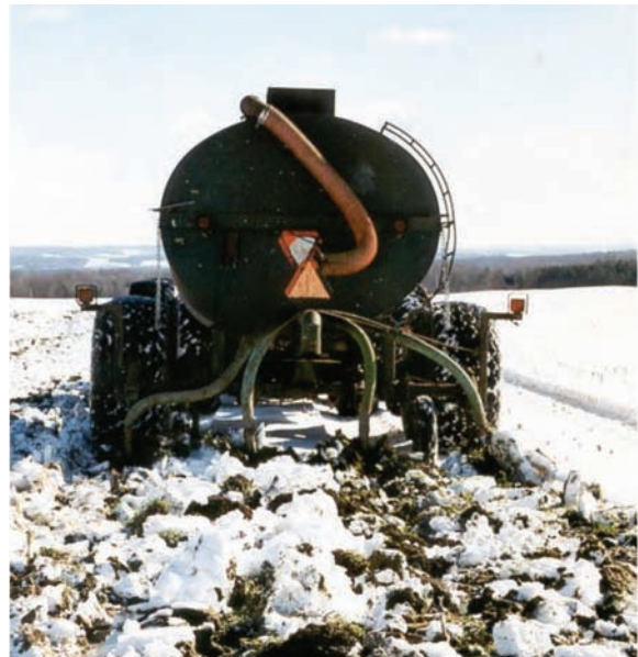
Figure 12.2. Injection of liquid manure into shallow frozen soils, which eliminates compaction concerns and reduces spring application volumes. Photo by Eleanor Jacobs.
