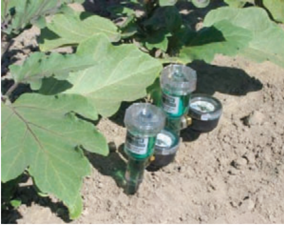
Figure 17.10. Tensiometers used for soil moisture sensing in irrigation management. Photo courtesy of the Irrrometer Company.
