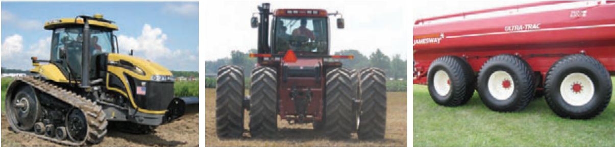
Figure 15.7. Reduction of soil compaction by increased distribution of equipment loads. Left: Tracks on a tractor. Middle: Dual wheels on a tractor that also increase traction. Right: Multiple axles and flotation tires on a liquid manure spreader
