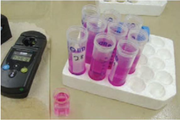
Figure 22.5. Assessment of active carbon using permanganate oxidation and a portable spectrophotometer. Photo by David Wolfe.
