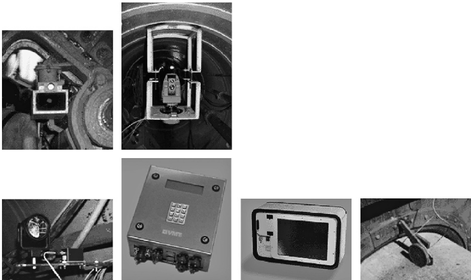
Figure 6-31 Components of the SLS-RV system from VMT GmbH. Top row from left: active target, laser theodolite. Bottom row: surveying prism, switching cabinet, control computer, measuring wheel; VMT GmbH.
