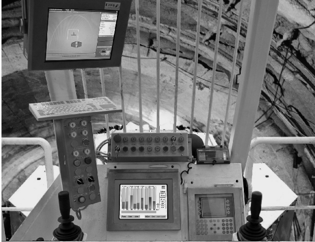
Figure 6-15 ALPINE MINER AM 105. Driver's cabin with display of directional control and the operating mode of the machine in December 2002.
