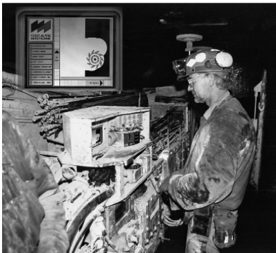
Figure 6-16 Visualisation of the cutting process of an ALPINE BOLTER MINER ABM 14 in the USA. The machine driver operates the machine by radio remote control and can observe the progress of cutting and the operational conditions on the display screen. The display, which the operator observes, is shown enlarged at top left.
