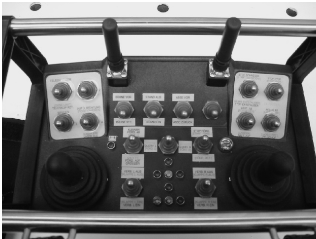
Figure 6-18 Radio remote control for ALPINE MINER AM 105 with return information.
