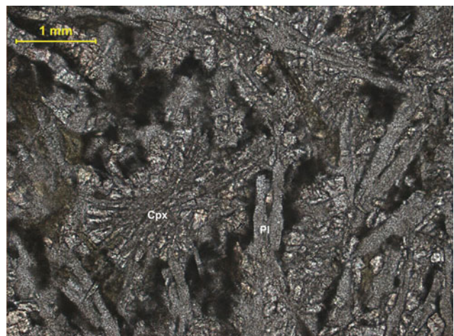
Plate V-4 Basalt 230/79-2 showing plagioclase laths and acicular sheafs of clinopyroxene. Small anhedral grains are epidote (230/79-8)
