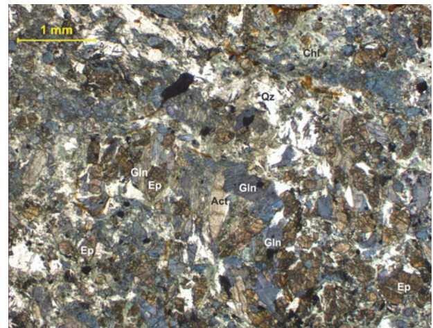
Plate Gln-41 Brecciated glaucophane schist consisting of phengite-rutile-zoisite-epidote-actinolite-glaucophane and traversed by secondary quartz and carbonate veins (N-146-6)
