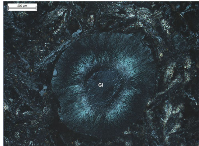
Plate V-8 Plagioclase-phyric basalt (V-7) between cross-polars showing spherule of glass with radiating fibres. The zoned spherulitic structure is developed at very high temperature (W11-4)
