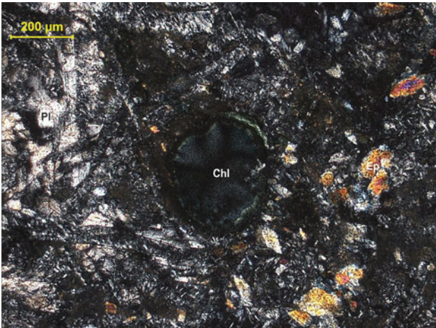
Plate V-6 Basalt (V-1) between crossed polars showing sectorial twinning in chlorite at the centre surrounded by granular epidote and laths of plagioclase (230/79-6)
