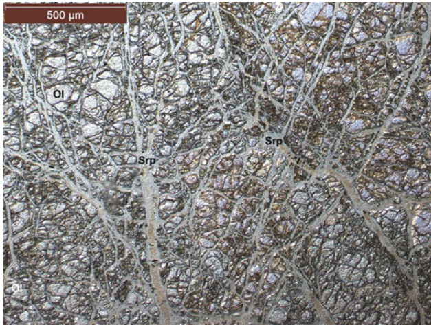
Plate PT-5 Fractured crystals of olivine in dunite traversed by serpentine veins cross-cutting each other (107/80-2)
