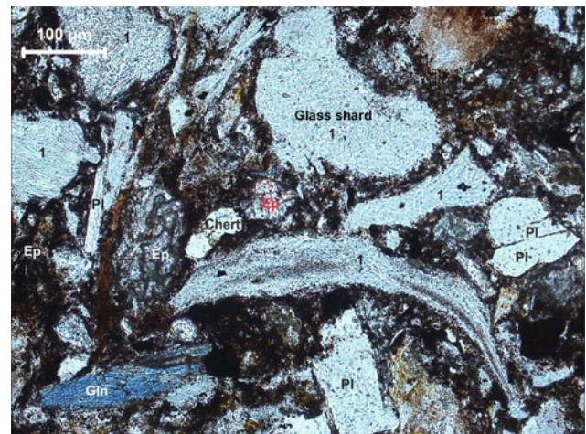
Plate Ptb-23 Tuff breccia between crossed polars showing poorly sorted angular lithic fragments of glass shards (1), chert, pleochroic blue amphibole (Gln), plagioclase (Pl) and epidote (Ep) (94/80-4)
