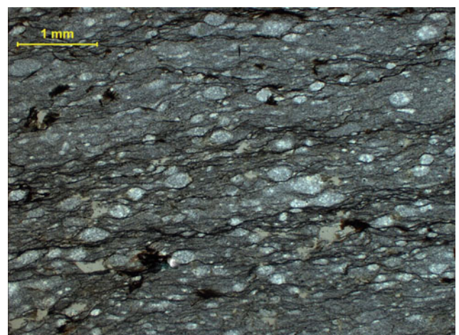
Plate OS_Ch-9 Tuffaceous chert showing radiolaria and fine biotite flakes along foliation. Crude crenulation is developed (Z55-1)
