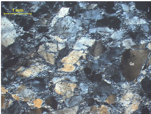
Plate OS_Sst-2 Feldspathic wacke between crossed polars showing tectonic foliation with development of a weak S-C fabric in the central part. Quartz shows anomalous extinction. Perthitic feldspar dominates over plagioclase (446/79-1)
