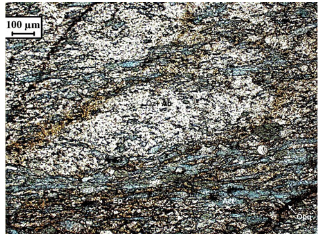
Plate GS-2 Finely foliated greenschist containing rows of brown epidote + green chlorite, and bluish green actinolite between quartzofeldspathic (albite) bands (43/80-1)
