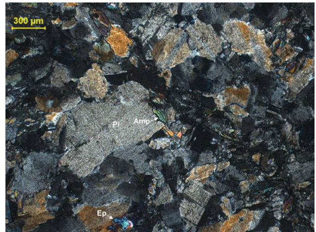
Plate PG-8 Diorite between crossed polars showing hypidiomorphic granular texture consisting of altered plagioclase, green amphibole and accessory epidote (K32-1)
