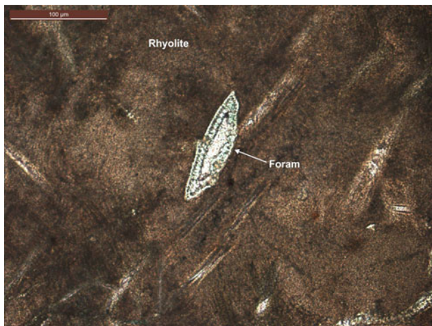
Plate Ptb-4 Magnified view of lenticular foraminifera (c, refers to Ptb-1) between crossed polars trapped in the rhyolite flow (C21/79-10)
