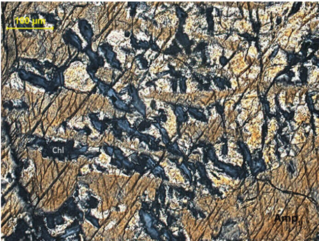
Plate An-5 High magnification view of poikilitic amphibole Amp_1 (magnesian-hornblende) in anorthosite T-74-3 between crossed polars showing alteration to chlorite (T-74-4)
