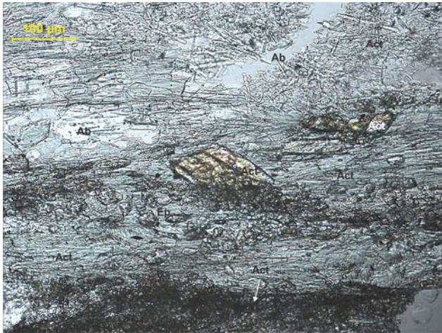
Plate OS_T-4 Magnified view of above rock (OS_T-3) showing actinolite needles at the centre and granular epidote below. The grey layer at the bottom is essentially composed of a mixture of actinolite and epidote. Rectangular ferroactinolite is pleochroic from pale greenish yellow to green (35-2)
