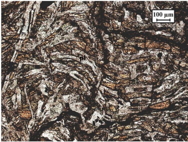
Plate Hy-11 Curved plagioclase and elongated brown clinopyroxene of mafic lava in fractured fragments of hyaloclastite showing intergranular texture (37/79-2)
