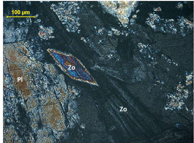
Plate An-7 High magnification view of rhombic and prismatic zoisite in anorthosite T-74 between crossed polars (T-74-8)
