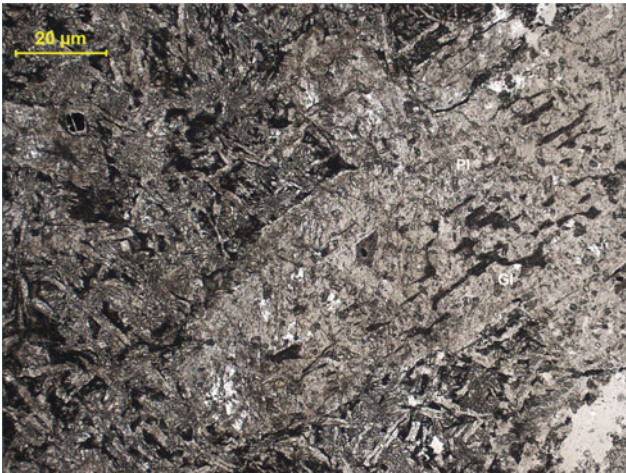
Plate V-5 Basalt (V-1) showing a large plagioclase phenocryst surrounded by a fine-grained groundmass with an intergranular to intersertal texture. Longitudinally aligned glass in plagioclase is developed along cleavage planes (230/79-9)
