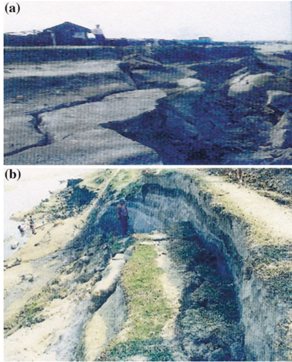
Plate 6 Rotated step like shear failure of the bank a - at neamighat, b - downstream of Nematighat
