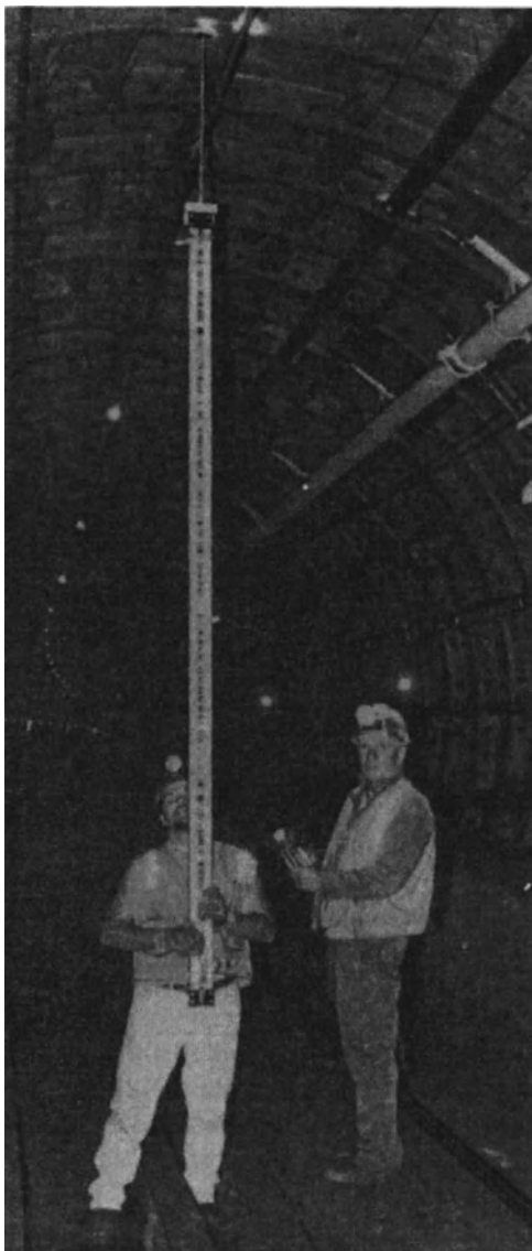
Fig. 3-35. Determining elevation of crown during deformation survey; note “bar-code” rod for automatic reading using Leica/Wild NA3000 level.
