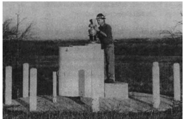
Fig. 3-5. DMT Gryomat 200. Gyrotheodolite mounted on primary horizontal control monument, Superconducting Super Collider project. (Photo courtesy Measurement Science, Inc.)
