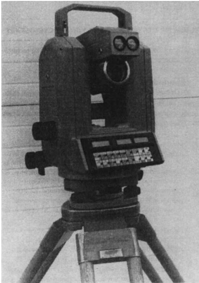
Fig. 3-1. Leica/Wild T2002 first-order theodolite with DI2000 distance meter (Total Station configuration).
