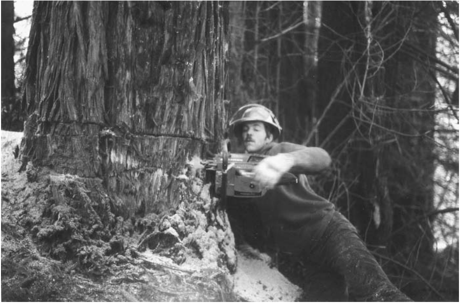
Photo 23 Aiming a tree to fall in a predetermined place is especially important in selective logging, where it is cost effective to minimize the impact on the forest and remaining trees. (Photograph by Walter Smith.)
