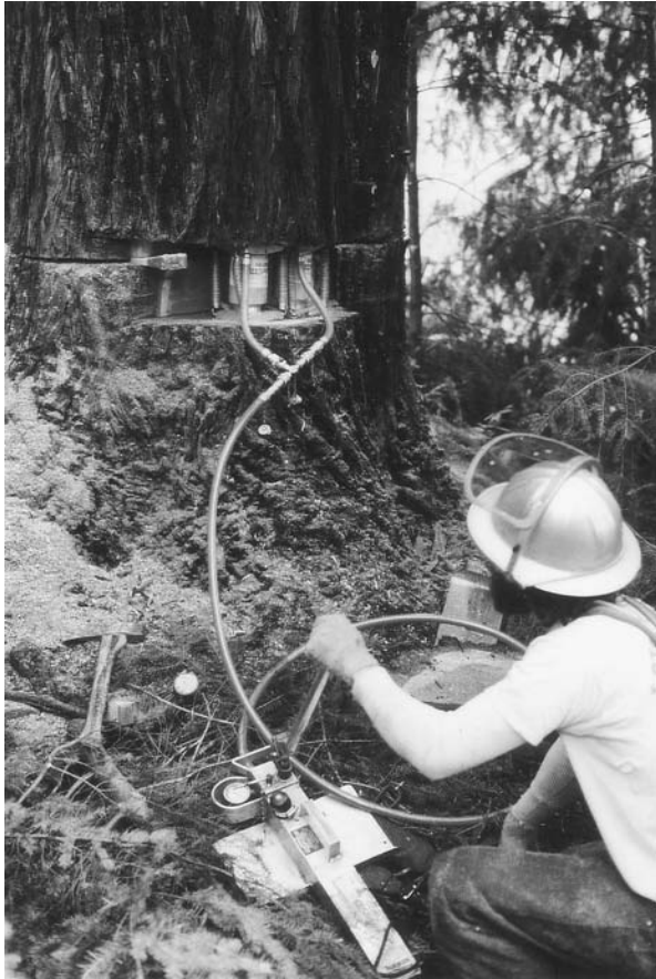
Photo 25 A feller using hydraulic jacks to fall a tree in the opposite direction of its lean. (Photograph by Walter Smith.)
