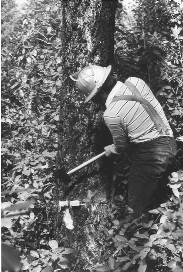
Photo 24 A feller using wedges to make a tree fall in the selected place. Note the hard hat and face shield. (Photograph by Walter Smith.)
