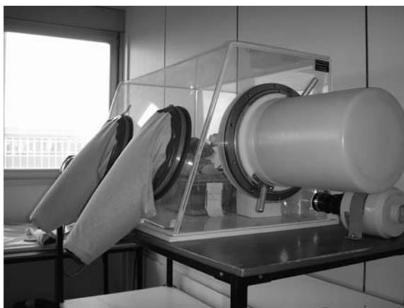
Fig. 15.1. Sterile isolator with its cylindrical transfer device.
