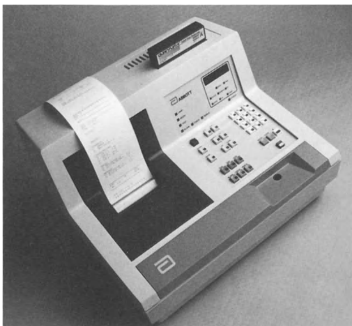
Fig. 24. Quantum I, a preprogrammed reader for single-tube ELISA tests which plots values and gives percent activity (Abbott Laboratories, Diagnostics Division, North Chicago, Illinois, USA)
