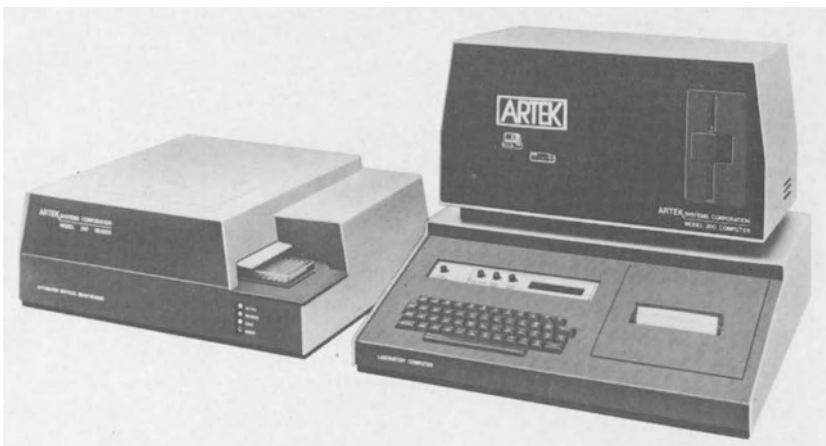
Fig. 22. The Artek Model 210 Reader and Computer, a computer-controlled reader with video display and printout. Data can be stored on disks and analyzed (Artek Systems Corporations, Farmingdale, New York, USA)
