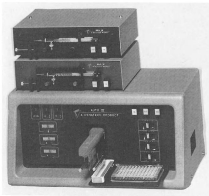
Fig. 9. The auto III with SRD III, an automated diluter, dispenser, and aspirator for microtiter plates (Dynatech Laboratories, Alexandria, Virginia, USA)
