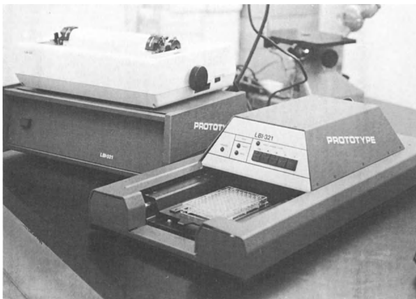
Fig. 23. The Bionetics Autoreader LBI-321, a programmable reader which scans eight microtiter wells simultaneously, and computer analyzes and prints the results; designed for the Bio-Enza Bead system. An automatic magnetic transfer device is also available (Litton Bionetics, Kensington, Maryland, USA)
