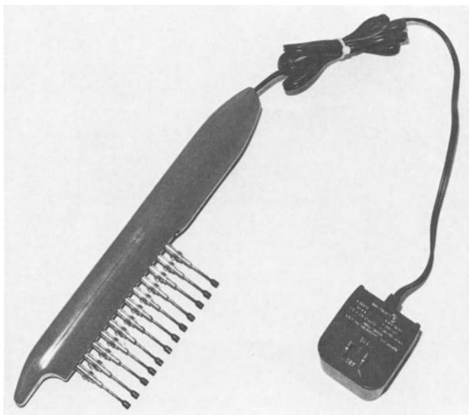
Fig. 8. The Rotatiter, a hand-held diluter for microtiter plates. "tulip" loop diluters are electrically rotated for serial dilutions (Dynatech Laboratories, Alexandria, Virginia, USA)
