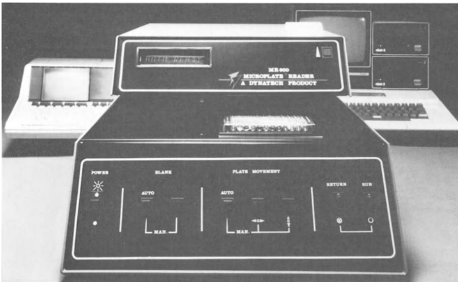
Fig. 20. Microplate Reader MR 600, a dual wavelength, automatic advance reader which can display and print results and can be linked with an Apple computer for data analysis (Dynatech Laboratories, Alexandria, Virginia, USA)
