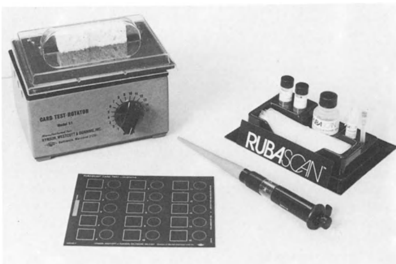
Fig. 26. Rubascan latex agglutination test, a 10-min card-agglutination test for rubella antibody. This rapid latex test avoids many of the steps required by other methods and can be performed easily in a physician's office, clinic, laboratory, or in the field (Hynson, Wescott and Dunning, Baltimore, Maryland, USA)
