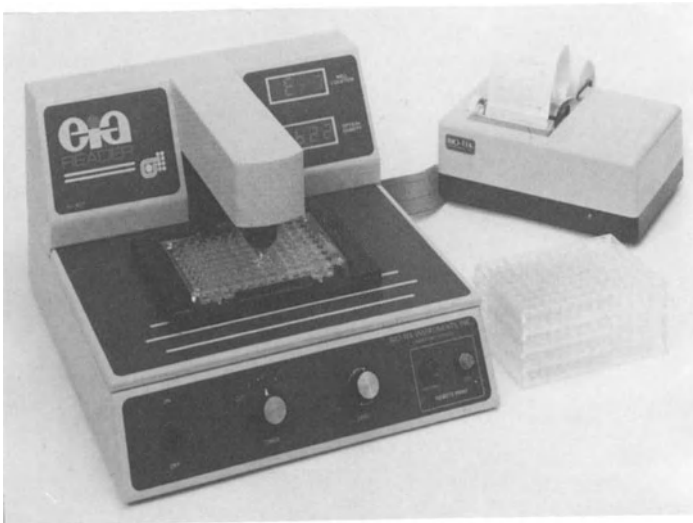
Fig. 19. EIA Reader Model 307. Plates are manually advanced and LED displays indicate optical density and plate position. An interface and printer are available (Bio-Tek Instruments Inc., Burlington, Vermont, USA)
