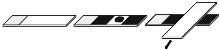
Fig. 3 Schematic diagram for preparing an agarose pad for microscopy. To a clean glass slide affix two pieces of tape. Between these spot 30 \mu l of molten 1% agarose and immediately cover with a second microscope slide. Wait for at least 20 min for the agarose to solidify. Pull the top slide towards you when ready to use. The agarose pad usually sticks to the top slide
