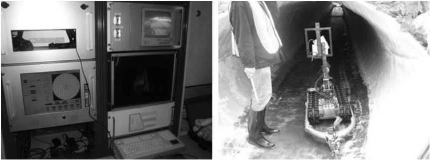
Figure 3-3. A Laser-Based Scanning System.
