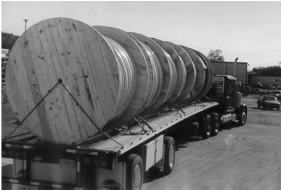
Figure 5-14. Reels of Folded Thermoplastic Pipeliners.
