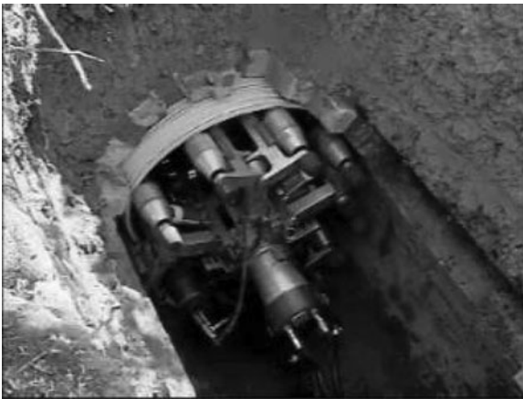
Figure 5-24. Traveling Winding Machine.
