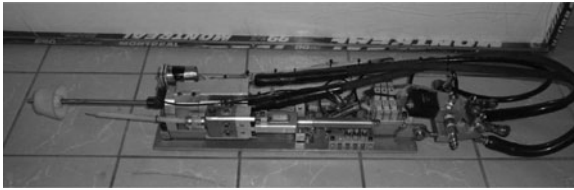
Figure 5-27. A Spray-On Robotic Unit for Coating Small Pipes.
