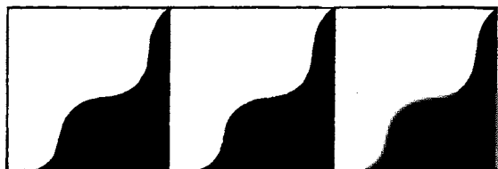
Fig. 15.18 Illustrating the formation of Mach bands. If this figure is rotated on a drum, at a rate above the critical fusion frequency, the subject sees a grey surface with alternate light and dark stripes, although there are no actual sharp transitions of luminance on the figure. (Graham, Vision and Visual Perception . John Wiley Inc.)
