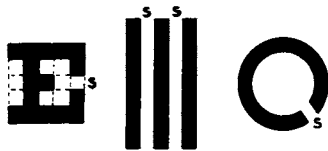
Fig. 7.7 Snellen letter, grating and Landolt-C. In each case the angle subtended at the eye by the distance, s , apparently determines whether the gap will be recognized.
