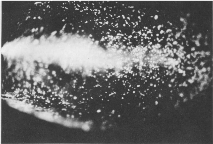
FIGURE 14.5 White crystalline deposits on the surface of a hydrogel lens due to heat disinfection in water containing minerals.
