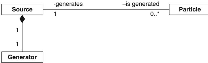
Fig. 15.2 Relations among the `Source`, `Particle` and `Generator` classes
