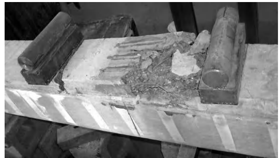
Figure 5 Failure mode of test specimen
