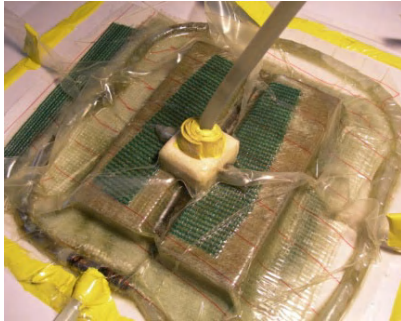
Figure 5 Manufacture process of grooved paulownia wood sandwich
