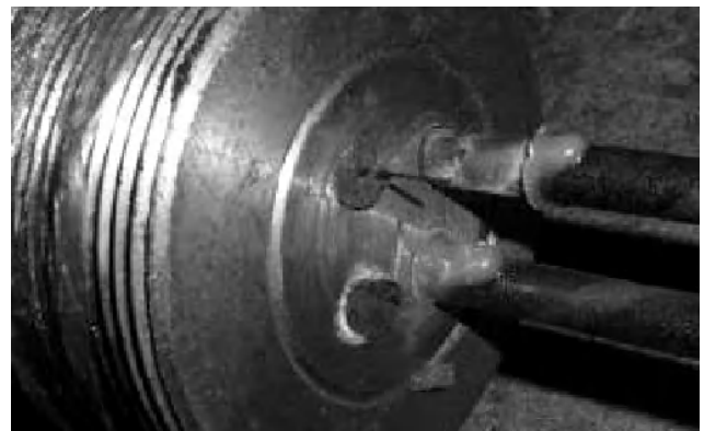
(a) Pull-out destruction and the CFRP tendons fractured just in front of anchor
