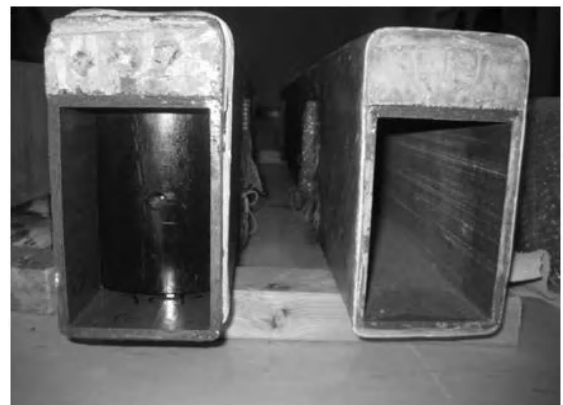
Figure 5 Support reinforcement with a plastic block
