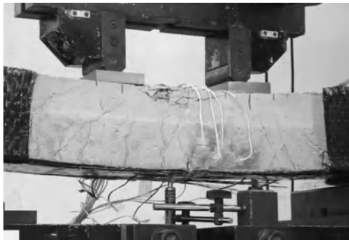
Figure 8 Failure of the CFRP strengthened RC beams
