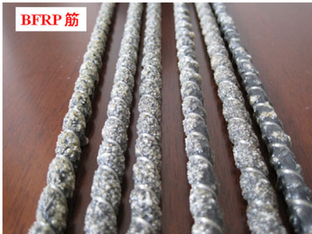
Figure 2 BFRP bar (nominal diameter, 8mm) tested in the present study
