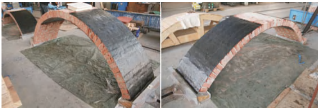
Figure 2 The barrel vault strengthened with CFRP in the area of tensile stresses
