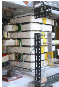
Photo 1 Retrofitted column specimen
