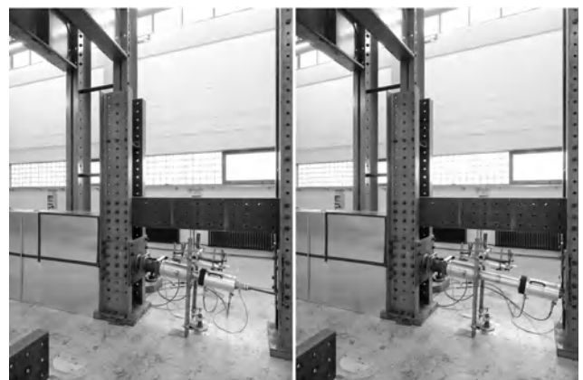
Figure 7 Setup of the hydraulic stressing jacks
