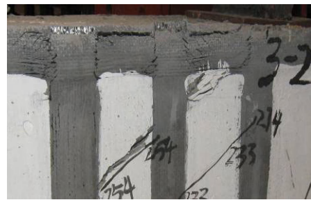
Figure 3 The shear debonding failure pictures
