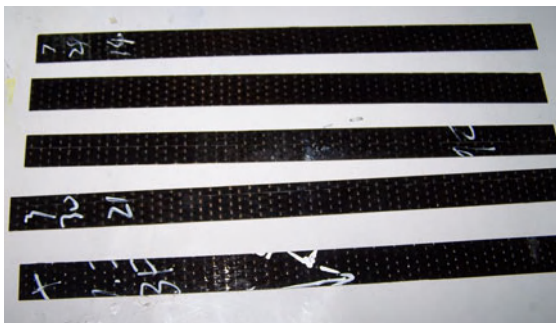
Figure 1 BFRP strips used for tensile testing
