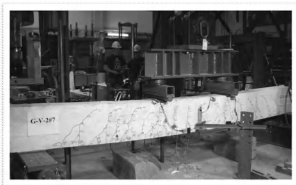
Figure 3 View of beam during testing (Beam G-V-2#7)
