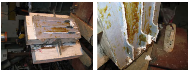
Figure 4 Shear failure on ribs of perfobond shear connectors
