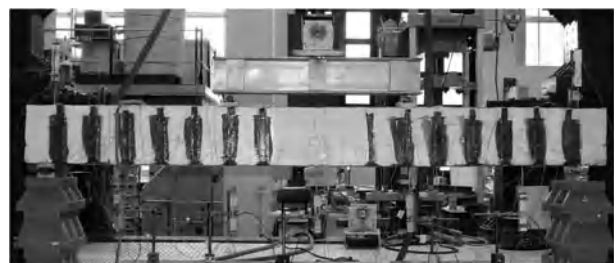
Figure 1 RC beam strengthened in shear with BFRP strips
