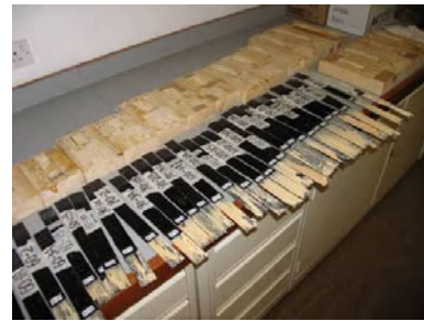
Figure 10 Debonded FRP plate and timber interfaces
