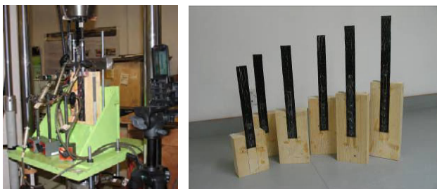
Figure 9 Single-shear FRP-to-timber joint tests
