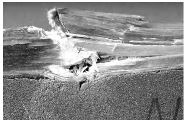
Figure 3 Typical compressive failure in unidirectional top flange. Picture taken from longitudinal cross section of girder No.1
