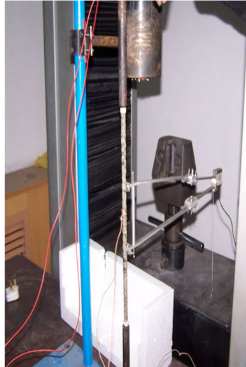
Figure 2 Thermocouple probes and high-temperature extensometer fixed to the rebar
