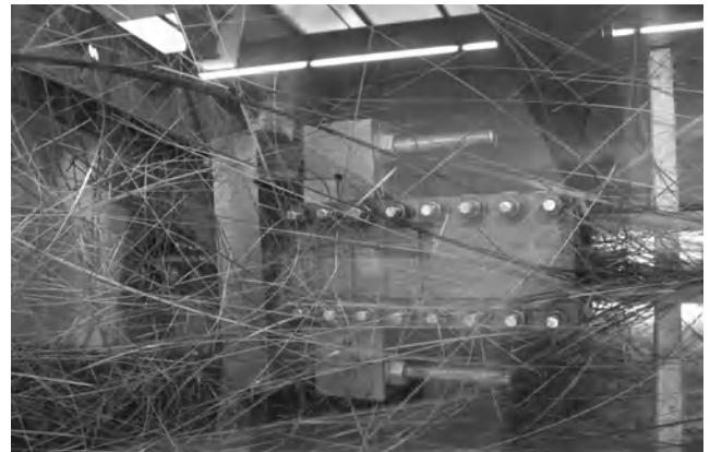
Figure 10 The end failure shape of the CFRP-strip
