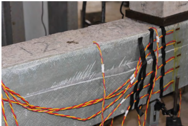
Figure 3 Beam FB2 after test: shear mode of failure is visible
