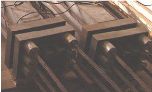
Figure 2 Anchorages and clamps for applying prestress to the CFL and RC beams
