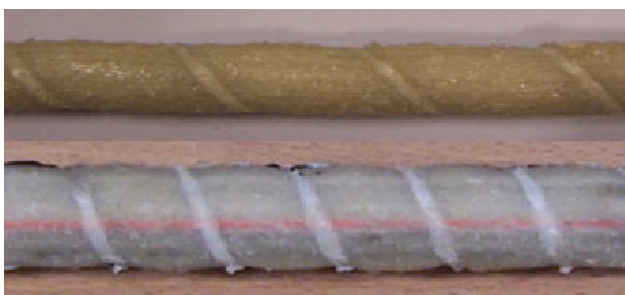
Figure 2 Helical wrapped GFRP rebar
