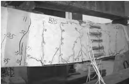
Figure 1 The middle debonding failure picture
