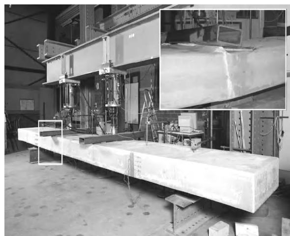
Figure 2 Shear wrinkling failure of web and subsequent failure of upper face sheet of GFRP sandwich beam subjected to four-point bending (Keller et al. 2008)
