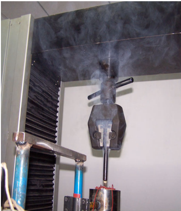
Figure 3 Smoke comes out from kiln at 200°C
