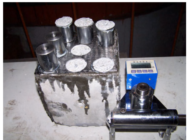
Figure 5 Pull-off testing of BFRP-concrete block with a pull-off testing machine on the left bottom
