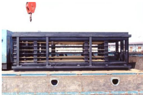
Figure 2 Steel frames for exposure test using six FRP cables
