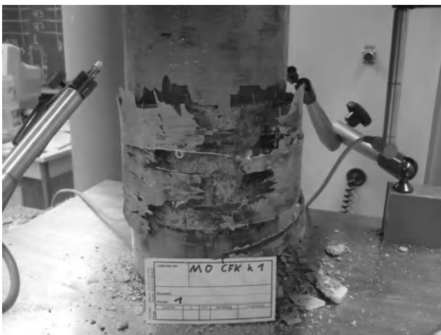
Figure 2 Short concrete column confined with CFRP sheets after failure
