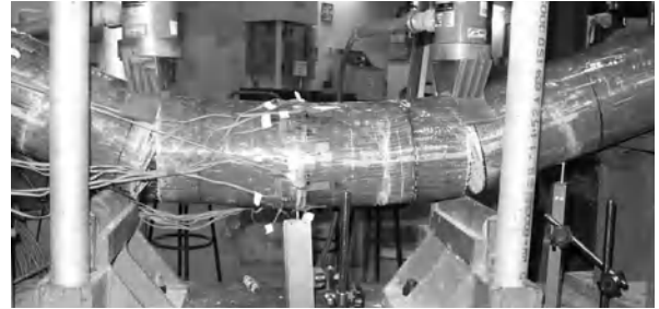
Figure 2 Failure of hybrid FRP-concrete-steel column (Yu et al., 2007)
