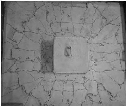
Figure 4 Typical crack pattern of test specimen (G450-18#20B) at failure
