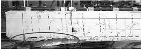
Figure 2 Rip-off failure of the control beam
