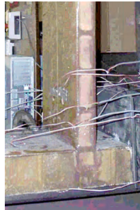
Figure 3 Unstiffened connection design
