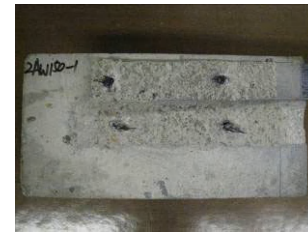
(c) Anchor rupture
