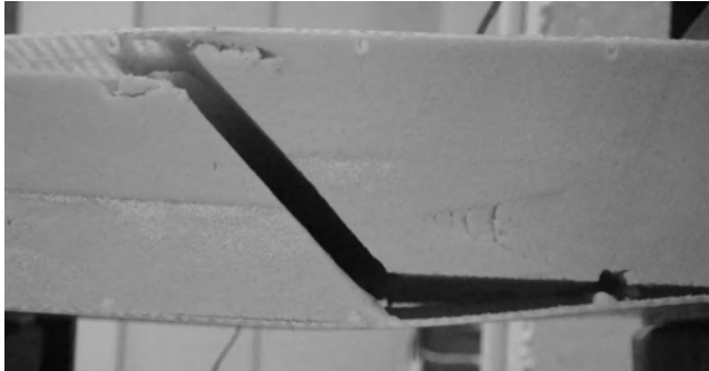
Figure 4 Shear failure at end of cycles
