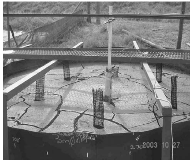
Fig. 9 Large-scale test of in-situ consolidation of mineral sands tailings
