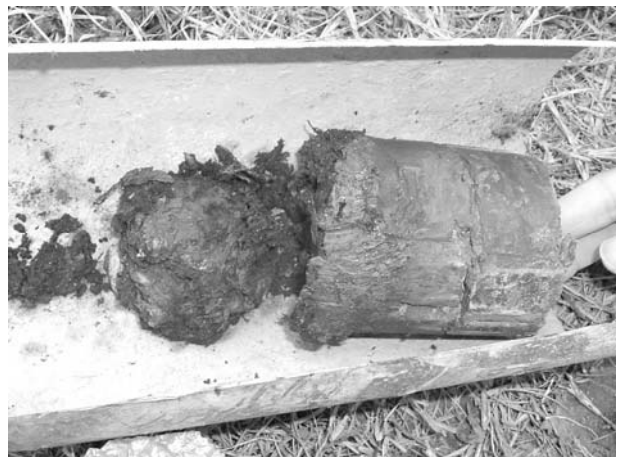
Fig. 6 Picture showing the first soil sample taken at the base of the landfill and in BH1
