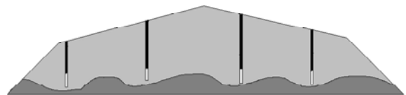
Fig. 6 Schematic section of a landfill with improved deep gas collectors at the end of the aftercare phase
