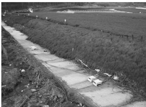
Fig. 23 Field trial windrow, sludge phyto-conditioning in the foreground, conventionally treated windrows in the far left.
