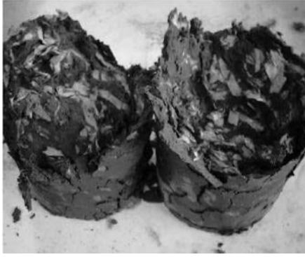
Fig. 10 Failure surface of cement stabilized pond sediment mixed with shredded paper
