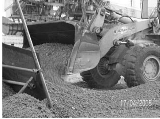
Fig. 2 Production of Hi-Beads at electrical power plant in Japan
