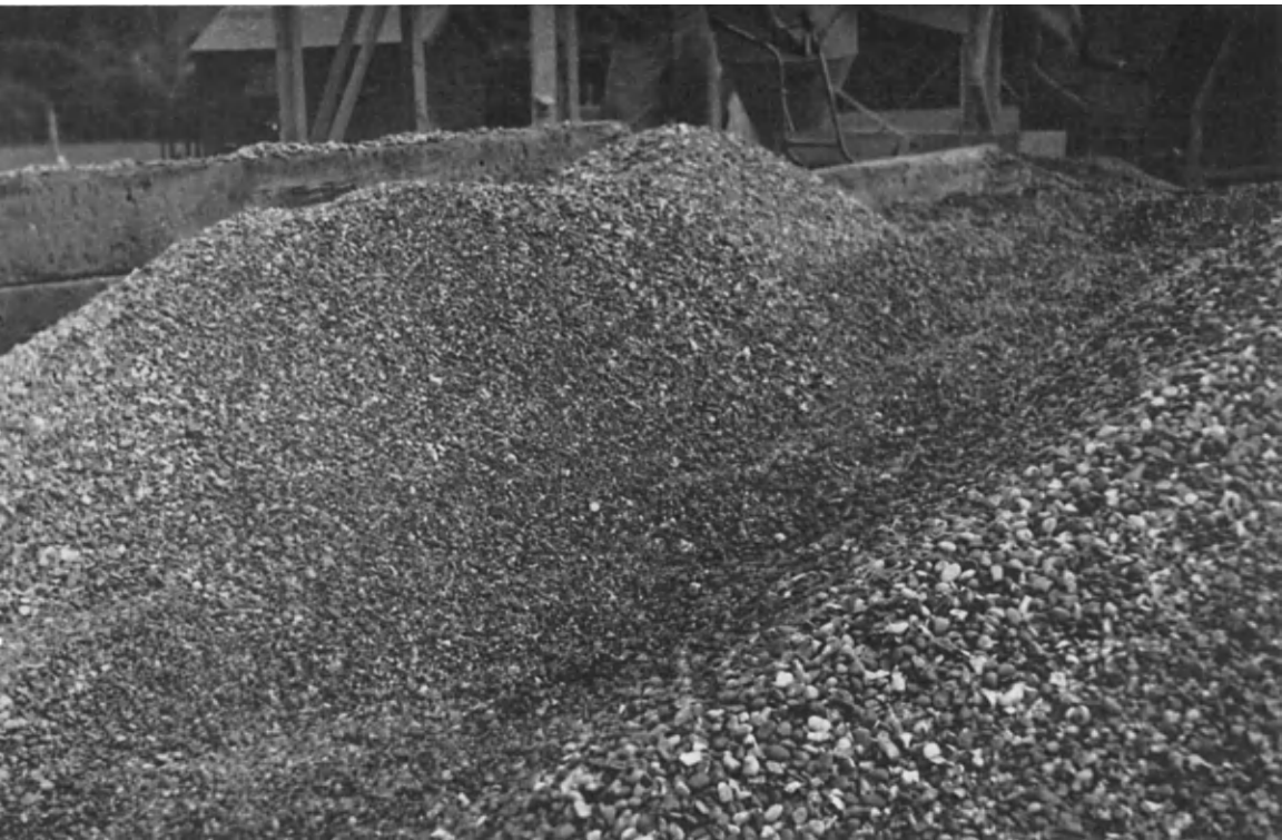
FIG. 2. A graded aggregate \frac{3}{4} – \frac{3}{16} in. showing poor mixing. The use of two separate sizes— \frac{3}{4} – \frac{3}{8} in. and \frac{3}{4} – \frac{3}{16} in.— is preferable.
