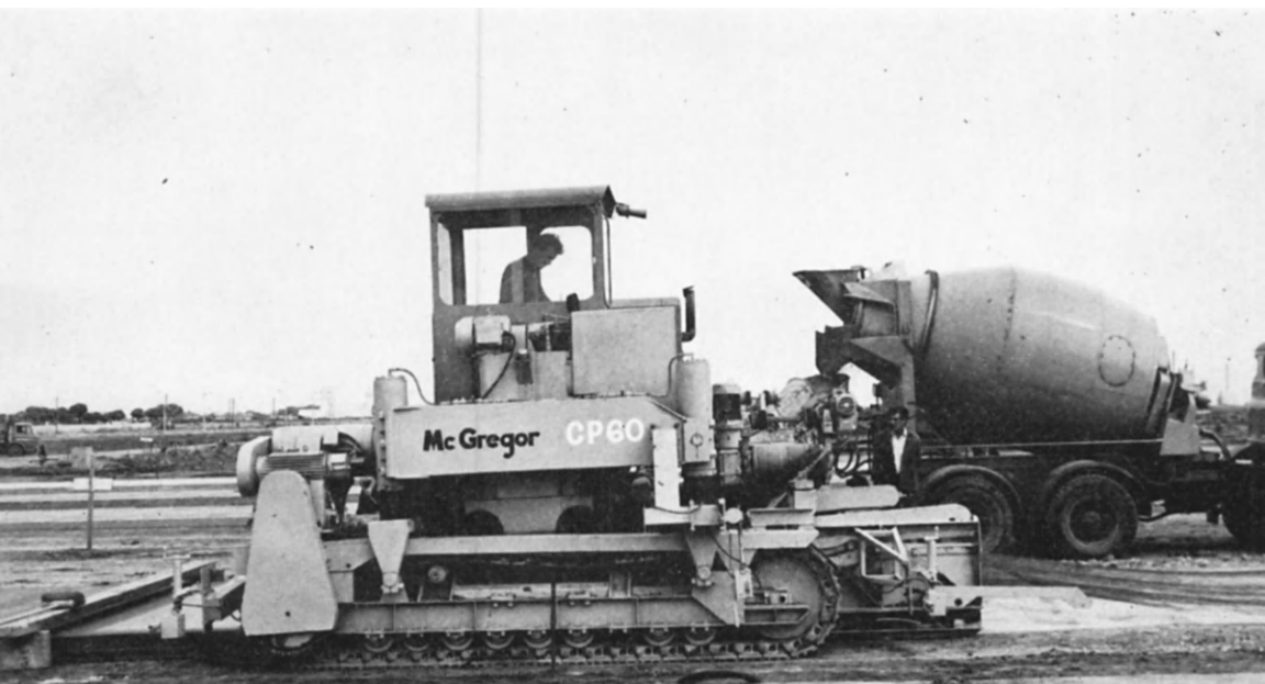
FIG. 43. A British slip form paver.
