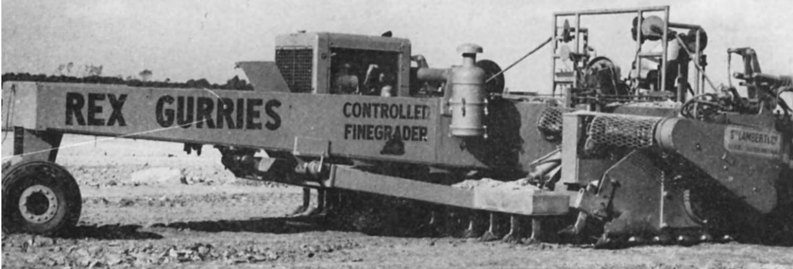
FIG. 25. A wire-guided grader for trimming earthworks, sub-bases or bases to fine limits.
