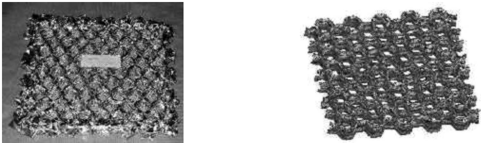
Figure 11.3 Crushing of honeycomb, test and simulation.
