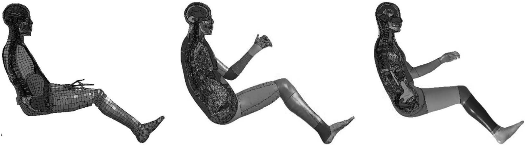
Figure 14.4 Mid-size male models, cut in the sagittal plane to visualize the internal structures: THUMS v3 (TMC 2008), THUMS v4 (Watanabe et al 2011), GHBMCM (Vavalle et al 2013).
