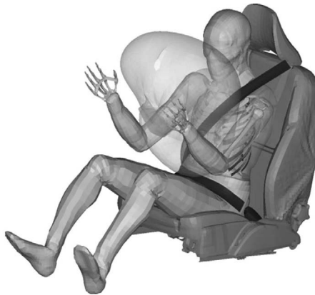
Figure 14.2 A finite element simulation of a frontal crash to analyze the thoracic injury risk for an occupant loaded by seat belt and airbag, here visualizing the shear stress in the ribs with THUMS (TMC 2008). Reprinted from (Mendoza-Vazquez 2014) with permission from Manuel Mendoza-Vazquez.
