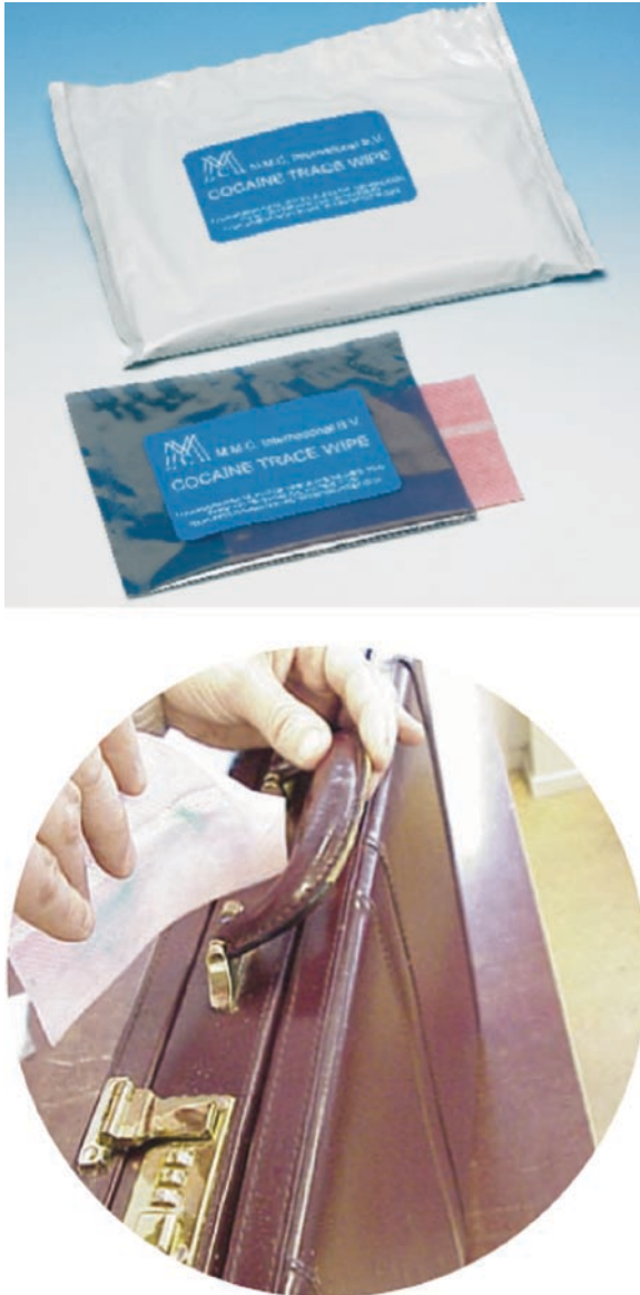
Fig. 27 The Trace Wipe Test for identification of cocaine smuggling or abuse
