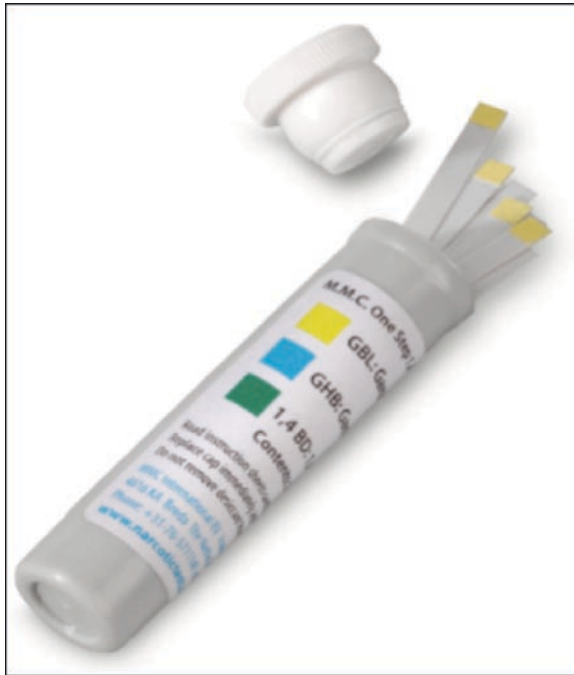
Fig. 13 The single test strip especially developed for identification of 1,4-butanediol, GBL, and GHB
