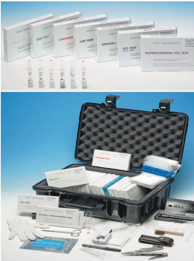
Fig. 29 Carrying vase with all necessary reagents to analyze unknown samples for illicit drugs
