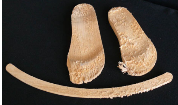
Fig. 8.2 Rejected wood products due to tension wood: wooden clog soles made from poplar and a clothes hanger made of beech, both showing expressed fuzzy grain surfaces
