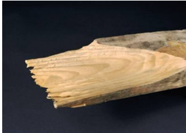
Fig. 9.3 Brash failure in lodgepole pine ( Pinus contorta Douglas) due to the presence of compression wood (reproduced with permission from Mochan and Hubert 2005 and covered by Crown copyright)
