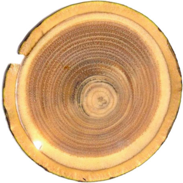
Fig. 9.1 Tension wood on the upper side of a leaning chestnut ( Castanea sativa ) stem (photograph courtesy of Bruno Clair, Université de Montpellier 2, France)
