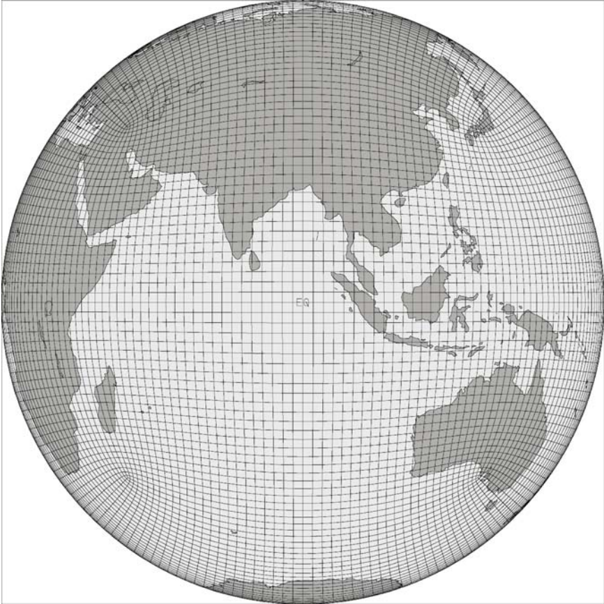
Fig. 4.1 A view of the CCAM C48 grid, having quasi-uniform resolution of 208 km
