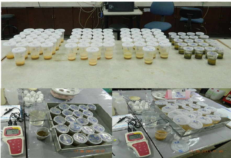
Fig. 7.12 Sample preparation procedures for pH test
