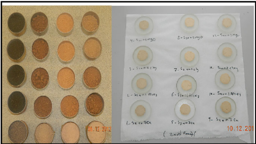
Fig. 7.14 Sample preparation procedures for XRD test
