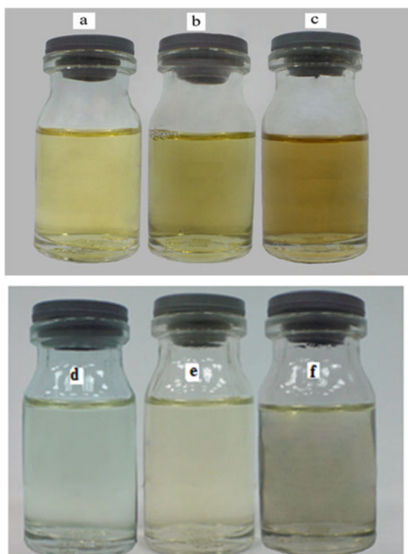
Fig. 18.7 The color change during time progression of the encapsulation between Zineb and MWCNT-g-PCA (a) initiated (b) after 2 h and (c) after 8 h and pymetrozine and MWCNT-g-PCA (d) initiated (e) after 2 h and (f) after 8 h
