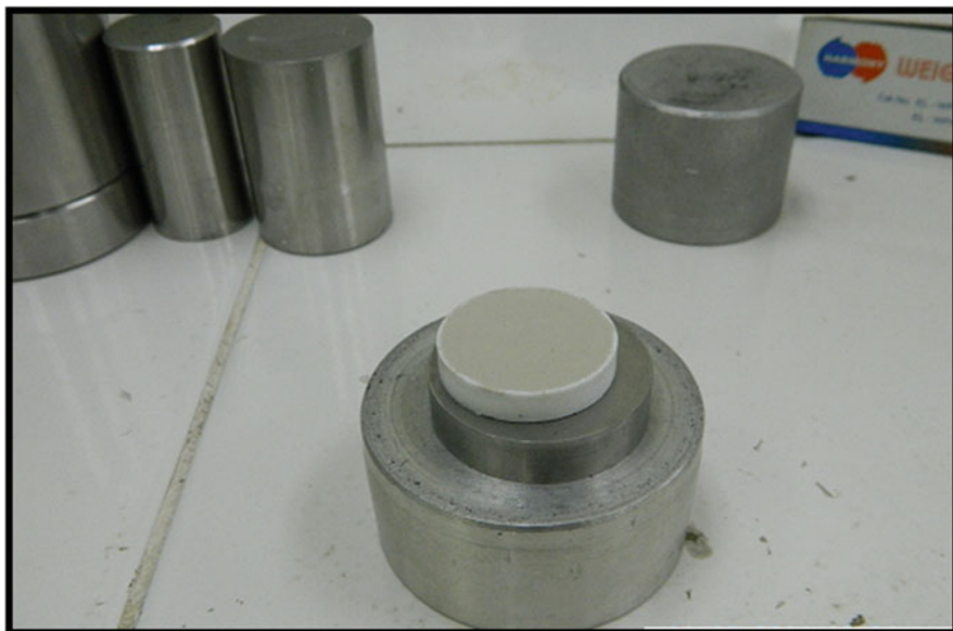
Fig. 7.16 Specimens prepared for XRF analysis
